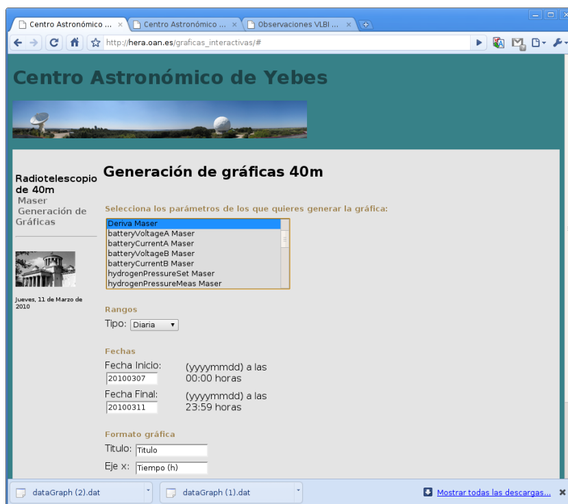
Figure 5: Web page at http://hera.oan.es/graficas_interactivas/ which allows to plot maser parameters as a function of time
