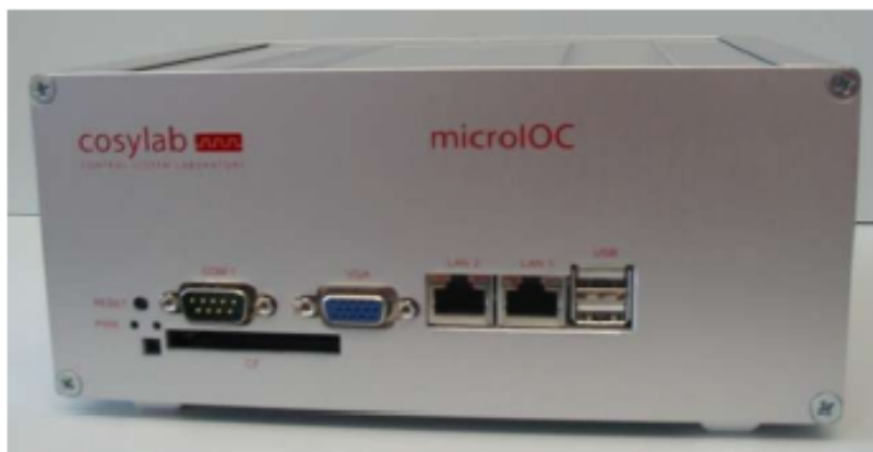
Front side of a microIOC in a small 2U enclosure.
