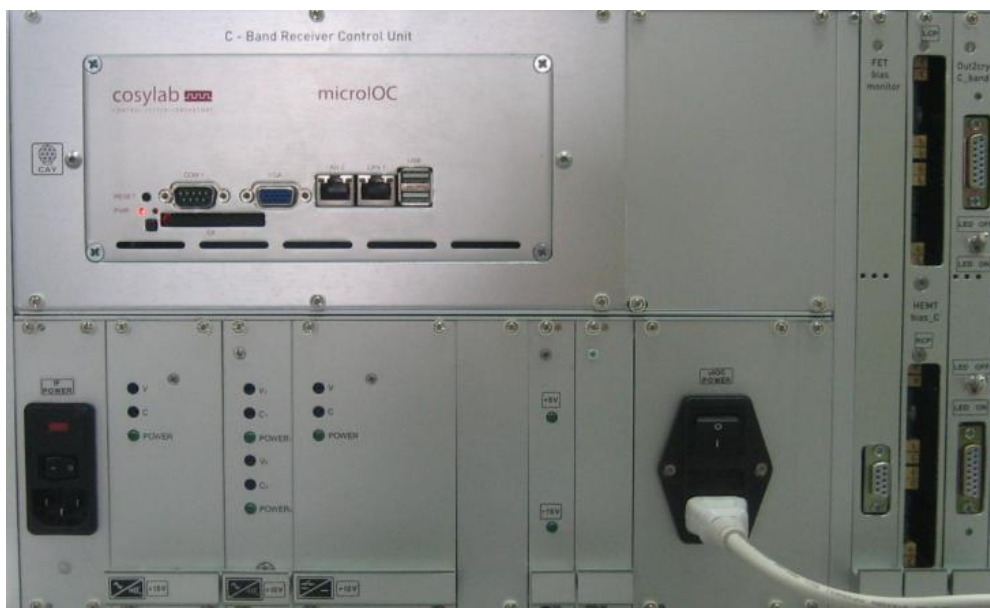
Figura 11: Receptor banda C
