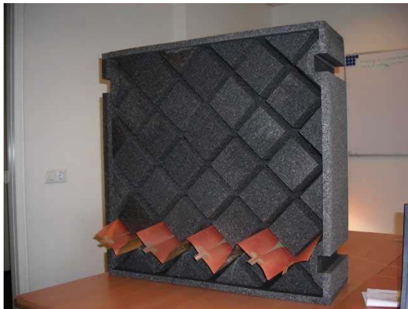
Figure 1: Foam structure for an array tile and polyester antenna elements.
