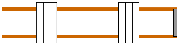
Figure 40: Differential load with Teflon support pieces (two equal spacing blocks).
