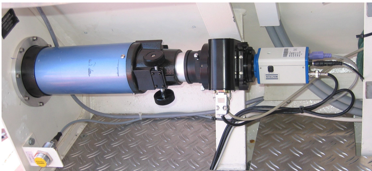
Figura 6: Photograph of the final mount prior to covering the telescope with a waterproof sleeve. .
