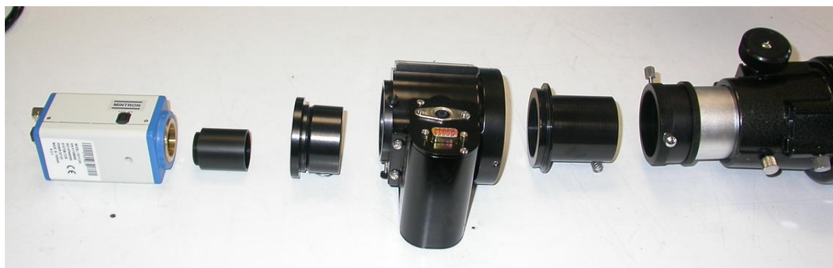
Figura 3: Photograph of the pieces that compose the optical telescope plus the focuser and the CCD camera. From left to right: Mintron camera (1 inch thread), 1 inch to 1 1/4 inch adapter, 1 1/4 inch to 2 inch adapter, Optec TCFS focuser, 2 inch Male Barrel, Skywatcher tube with 2 inch thread.
