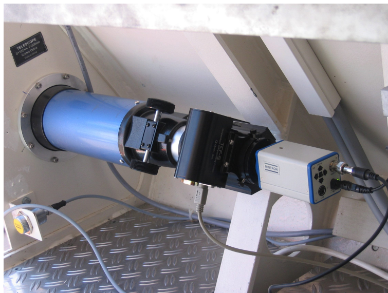
Figura 1: Photograph inside the subreflector cabin, where the telescope is housed. The size of the telescope is limited by the form of the wall, the girder and the rear metallic structure (hardly seen in the photograph). The camera was not upside down as with the definitive setup.
