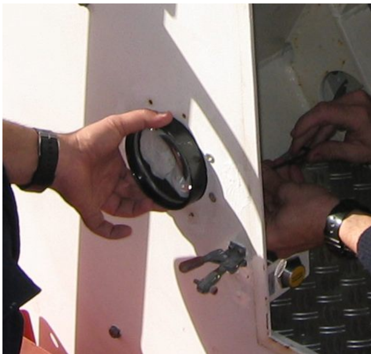
Figura 5: Photograph while screwing the metallic ring to the subreflector wall. The lens can be seen inside its cell. The outer end of the cell passes through the hole in the subreflector cabin wall and protrudes a couple of cm outside.
