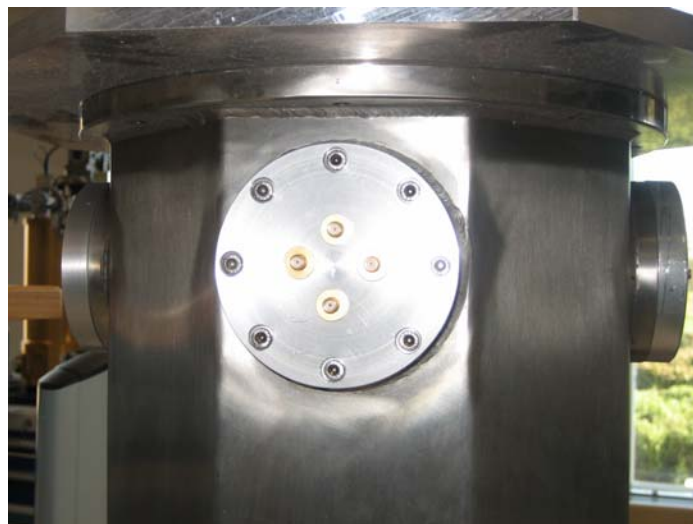
figura 23: Vista frontal del vacuum case
