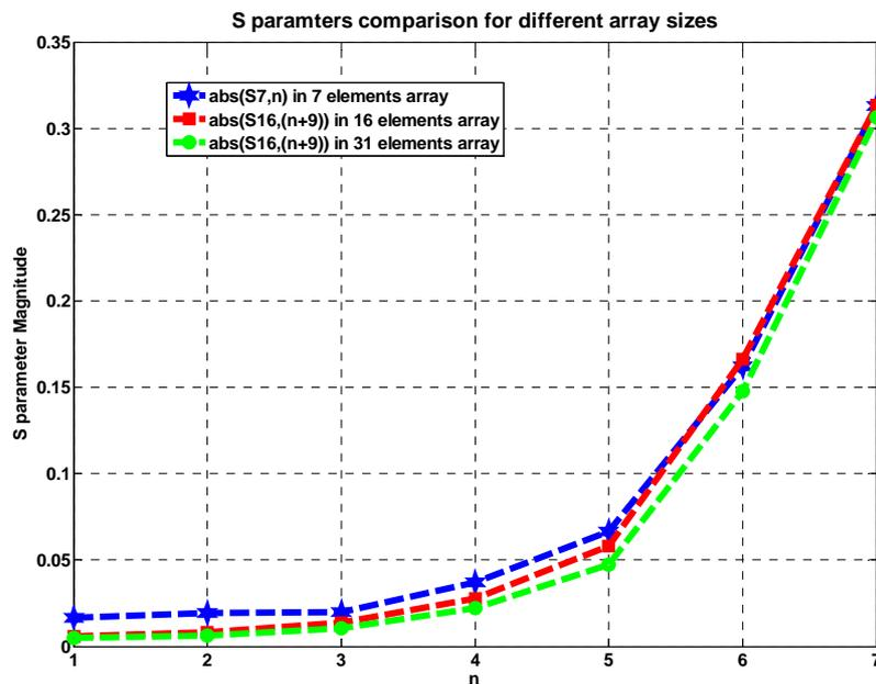
Fig. 4.4: S parameters magnitude comparison
