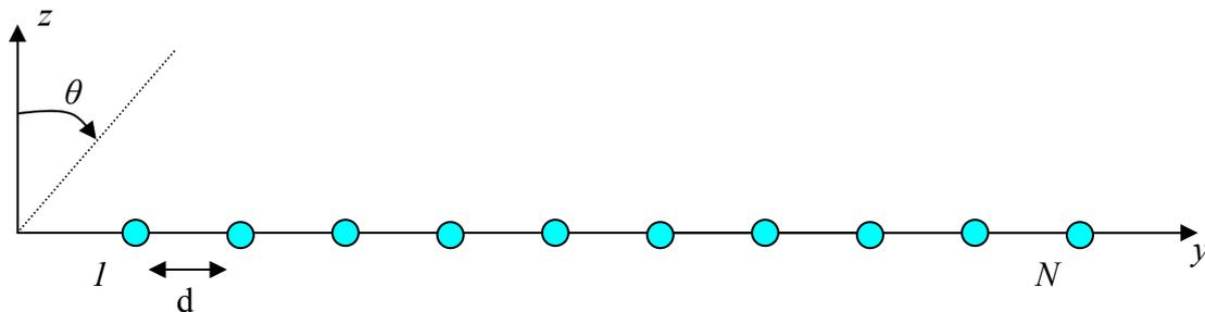
**Fig. 2.1: Linear Uniform Array of  $N$  elements**
