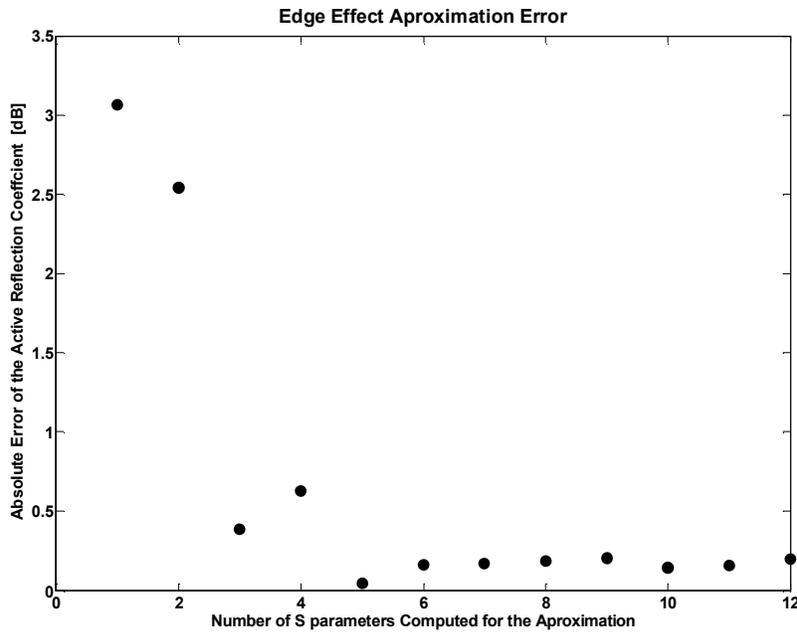
Fig. 3: Edge Effect Approximation Error for a 16 dipoles array
