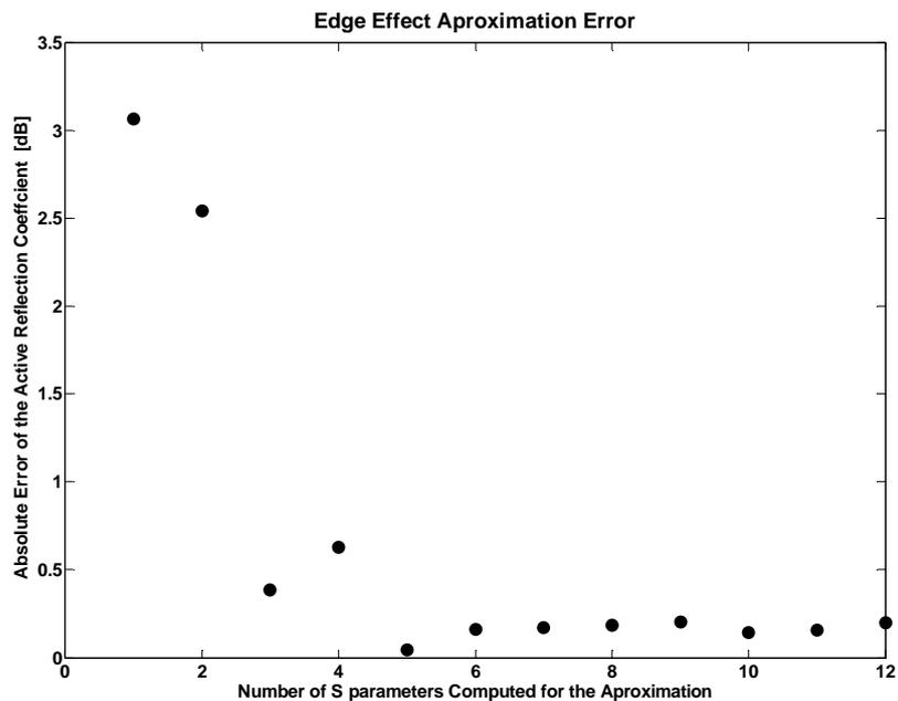
**Fig. 4.7: Edge Effect Aproximation Error for a 16 dipoles array**
