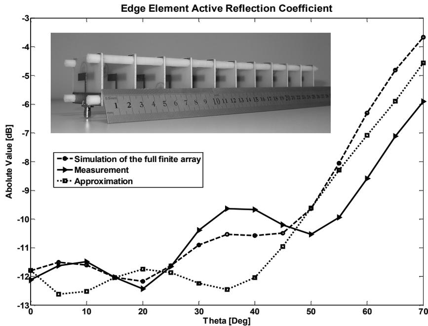
Fig. 4: Edge Effect Approximation for 11 Printed Dipoles Array
