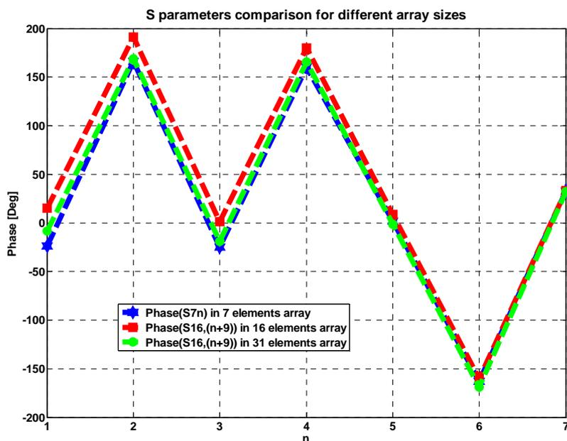
Fig. 4.5: S parameters phase comparison
