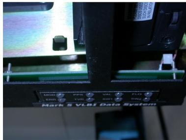
Figura 6: View of the front LED panel from upwards. Two long screws and its bolts can be seen. There are 4 screws in total. On the right the flat cable.
