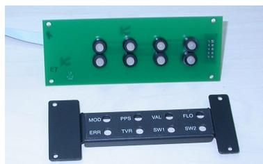
Figura 4: View of LED board, the black plate and the flat 10 wire cable
