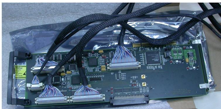
Figura 2: View of the withdrawn Mark5A I/O board with the cables which were connected to the Mark5A panel.
