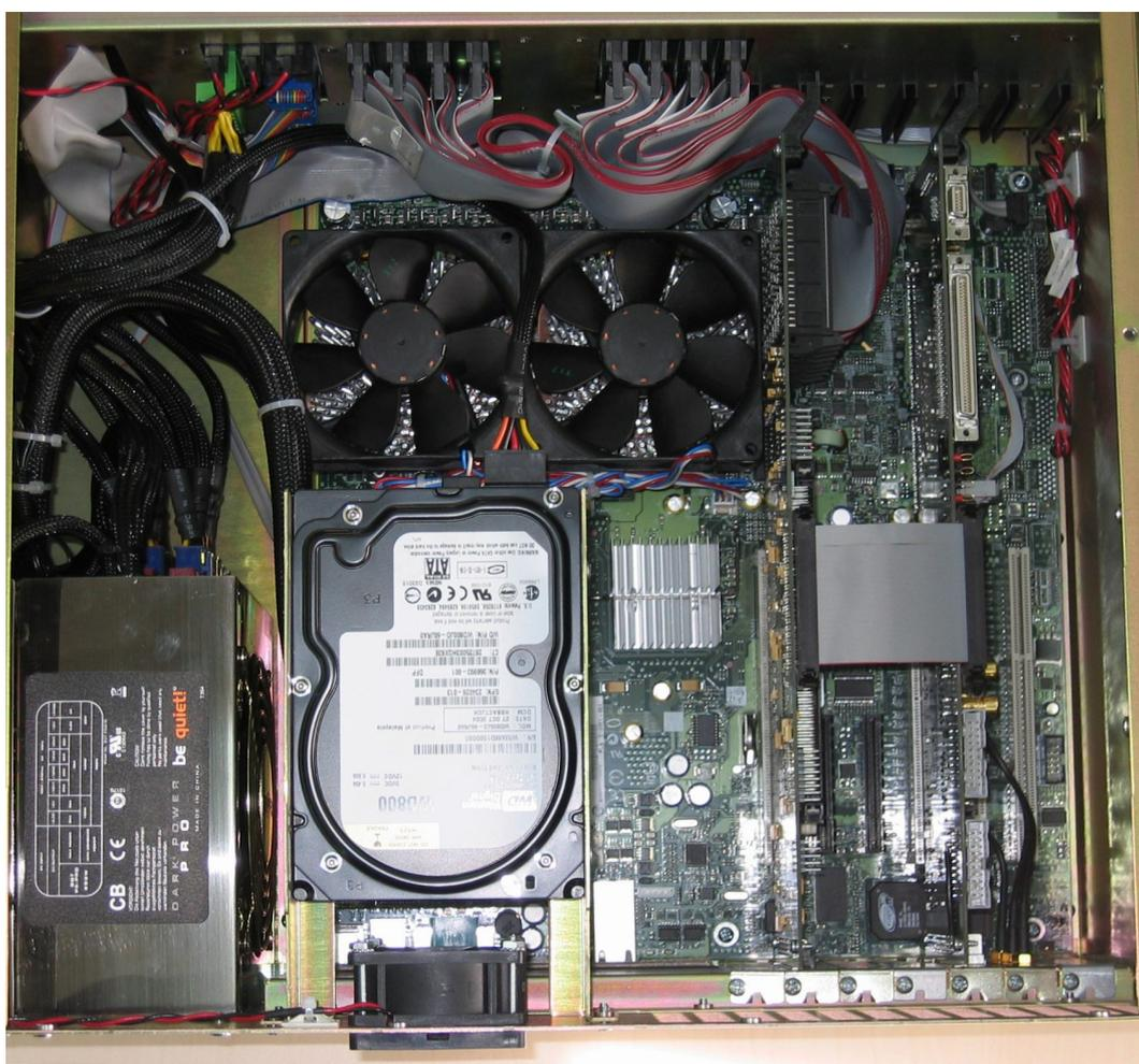
Figura 11: Image of the Mark5B once the upgrade was completed.
