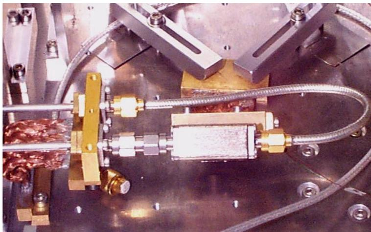
Figure 1: Isolator PAMTECH Inside test Dewar.
