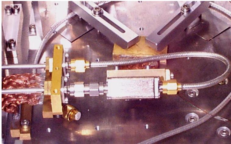
**Figure 1:** Isolator PAMTECH Inside test Dewar.
