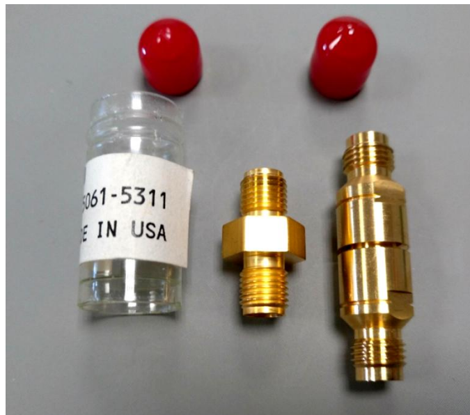
Figure 1: Photo of the transitions used to connect the power sensor to the port 1 of the PNA-X for power calibration. Left: a short 3.5 mm female to female PN 5061-5311 used for measurements up to 26.5 GHz. Right: metrology grade 1.85 mm female to female PN 85058-60114 (included with N4694A E-cal module)
