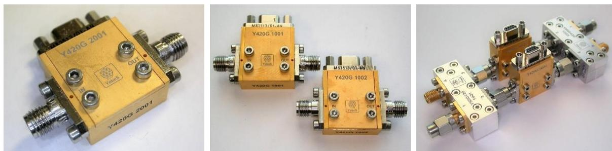
Figure 1: Amplifiers developed during the first two phases of the project. Y420G 2001 (baseline design and deliverable D 01) on the left. Y420G 1001 and 1002 (alternative design) on the center (sent to NOVA). Balanced amplifier (with 4-20 GHz hybrids) on the right.
