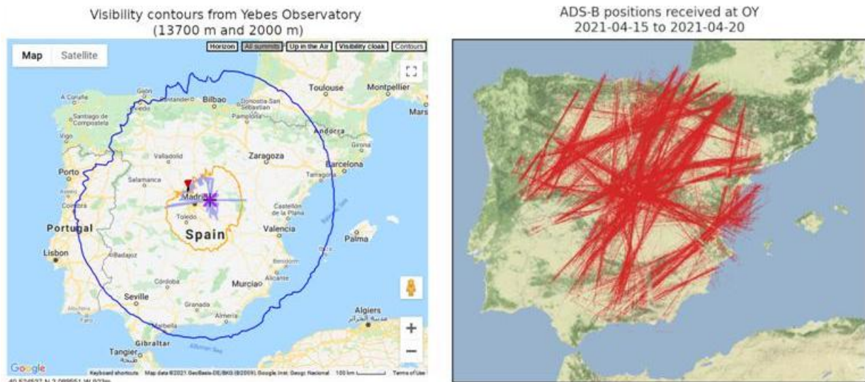
Figure 42. Geographical coverage of the ADS-B receiver from Yebes Observatory. a) Computed horizon line-of-sight contour at 2000 m (yellow) and 13700 m (blue). b) Actual coverage for a period of five days.
