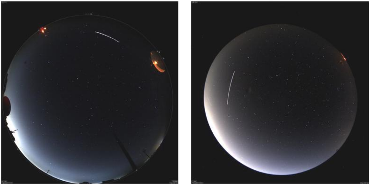
Figure 54. All sky camera: night images taken without (left) and with baffled (right) camera. A small part of the camera field of view is lost for the baffled option. Stars in the field are better seen due to the increase of contrast of the image.
