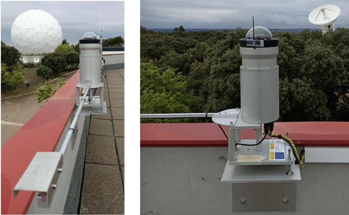
Figure 35. Outdoor installation: All sky camera.
