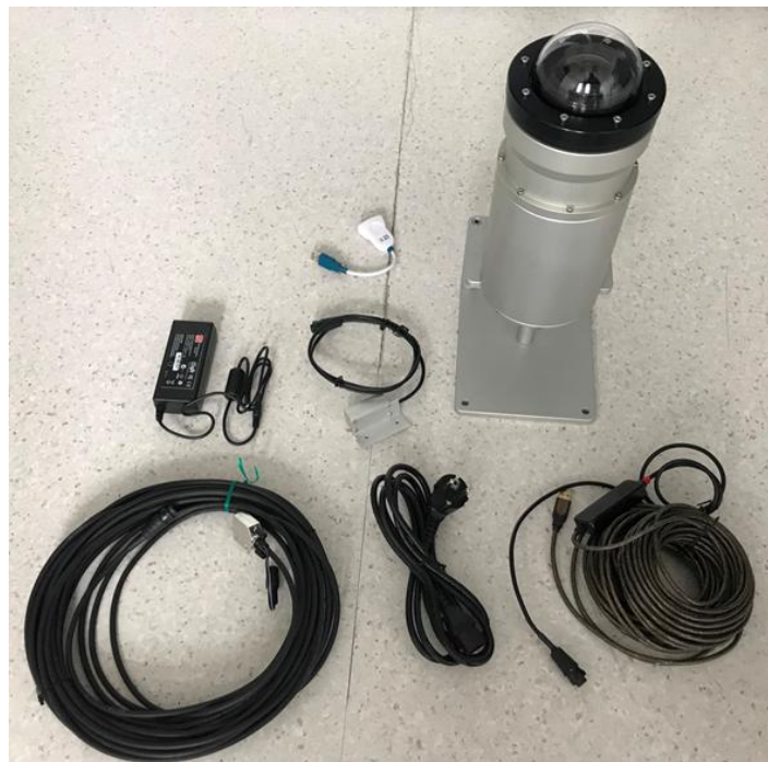
Figure 8. All Sky Camera: components.
