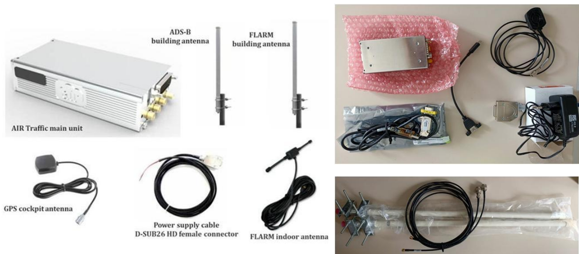
Figure 5. Air Traffic Receiver (FLARM): components.
