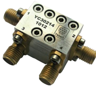
Figure 5. Photograph of the 30 dB directional coupler from Yebes.
