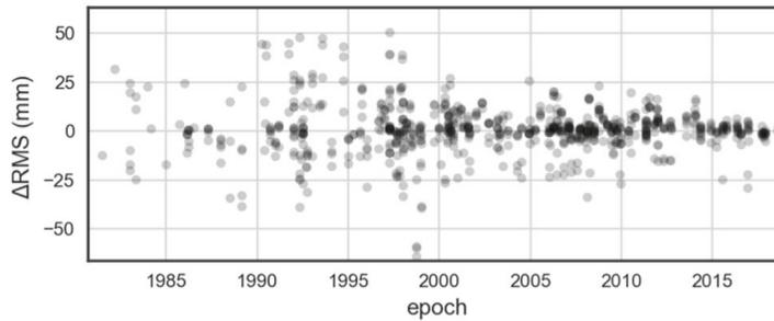
**Figure 2: Differences between the modelled and empirical NP RMS for the satellites and stations included in the first release of the CoM tables [1].**
