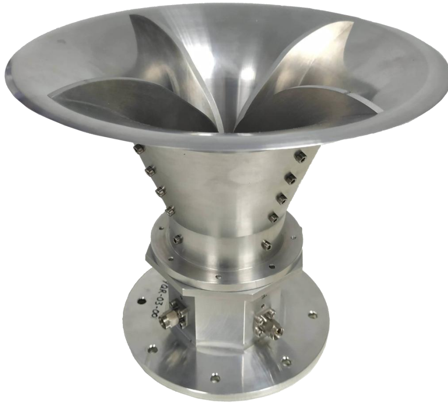
Fig. 1.1. Picture of the QRFH antenna.
