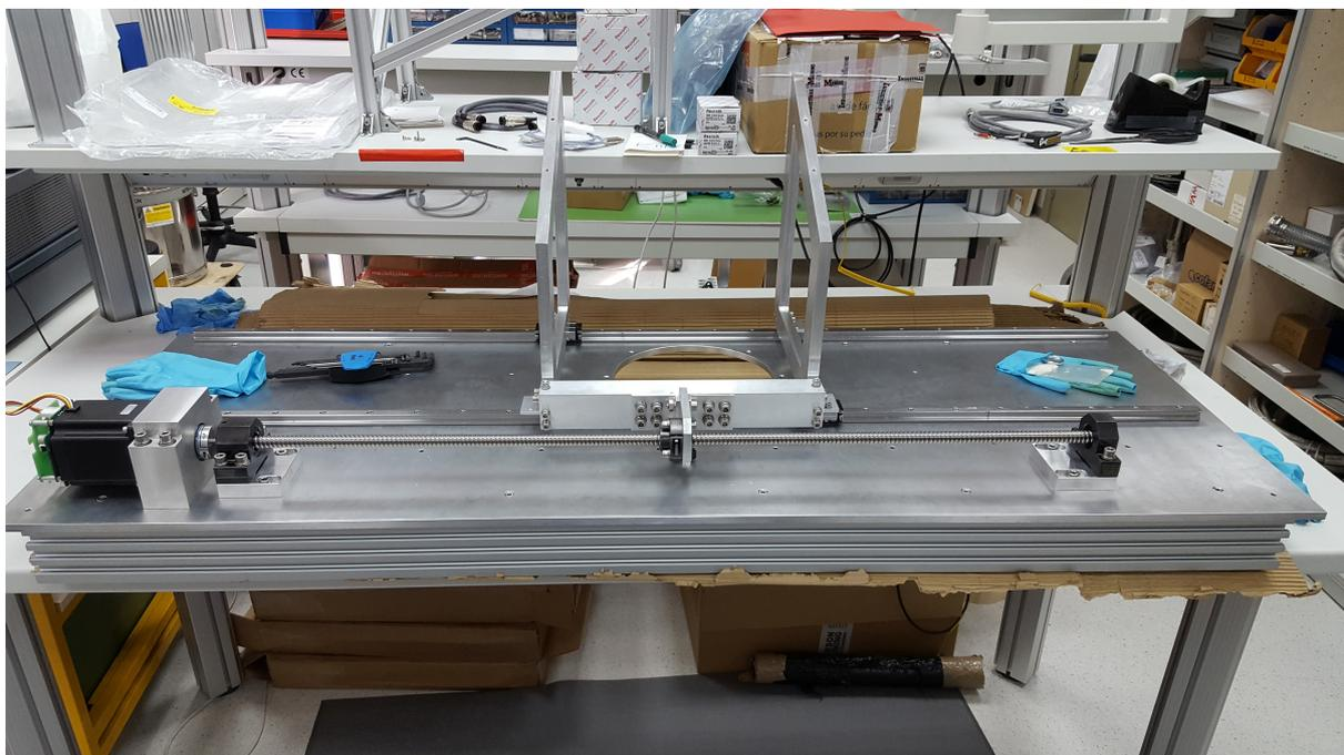
Figure 5.4: Partial assembly of the linear motion system with the load
