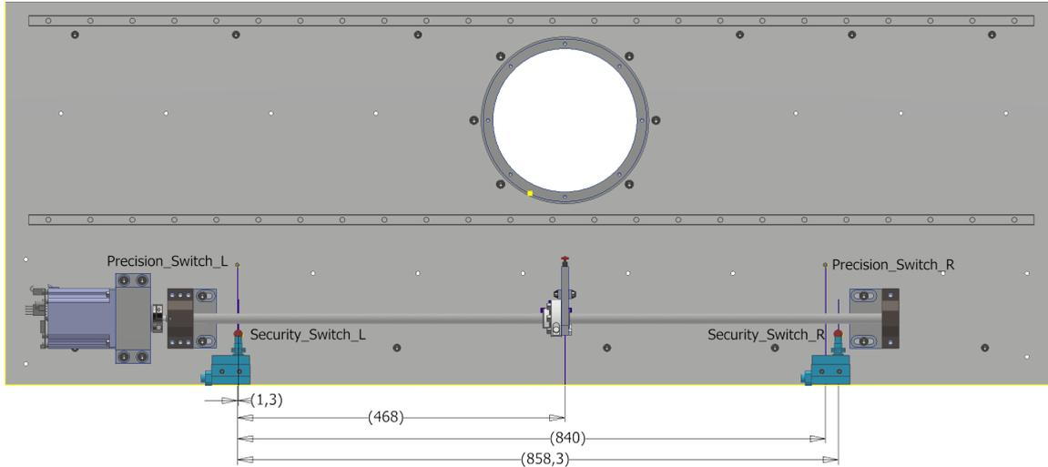
Figure 3.4: Switch position schematic
