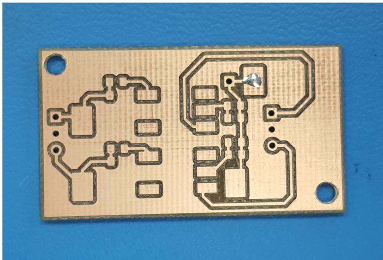
Figure 5.1: Switch Isolator PCB
