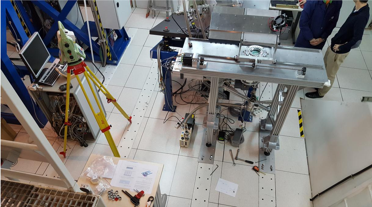
Figure 5.9: Alignment process with the total station
