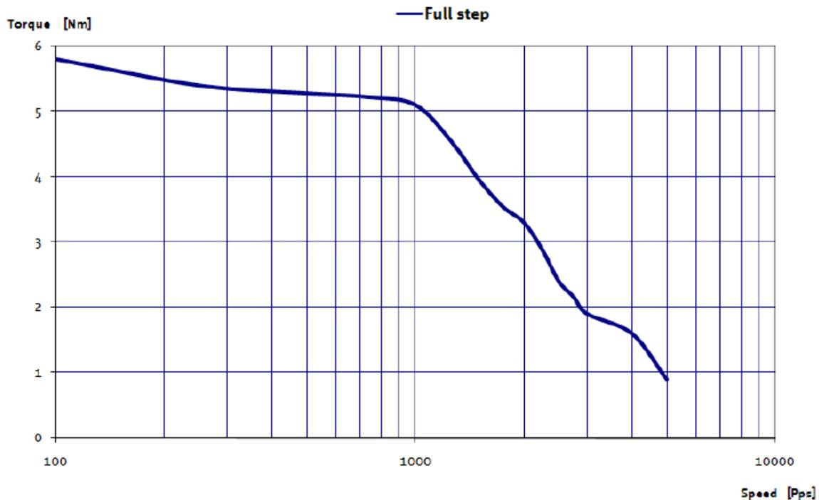
Figure 6.1: Speed vs Torque (micro-step per second)
