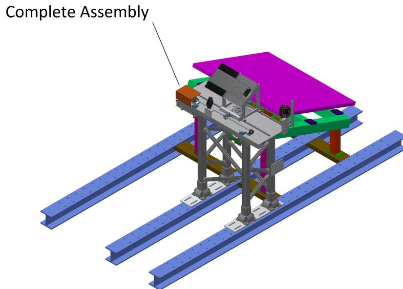
Figure 3.1: Complete assembly in the receivers cabin of the radio-telescope
