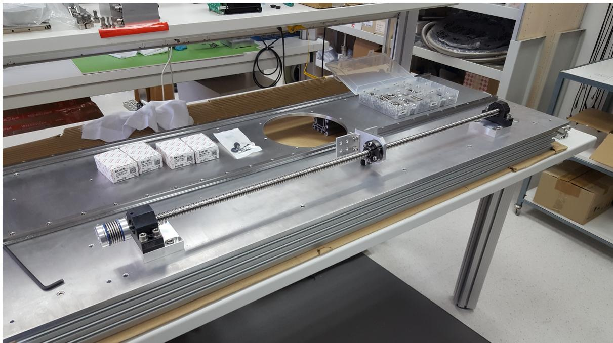
Figure 5.3: Partial assembly of the linear motion system
