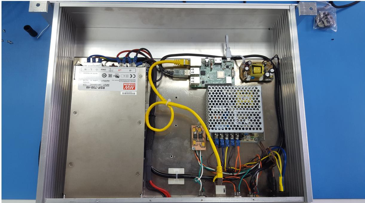
Figure 3.8: Power supply and control module
