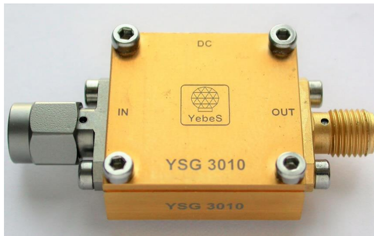
Figure 1: External view of a YSG 3 LNA. Dimensions excluding, connectors are 24×23×8.6 mm (X×Y×Z in the picture)
