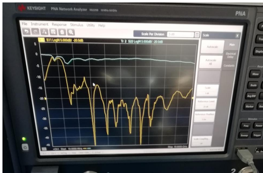
Fig. 3.1. Measured reflection coefficient showing high reflection in port 1.
