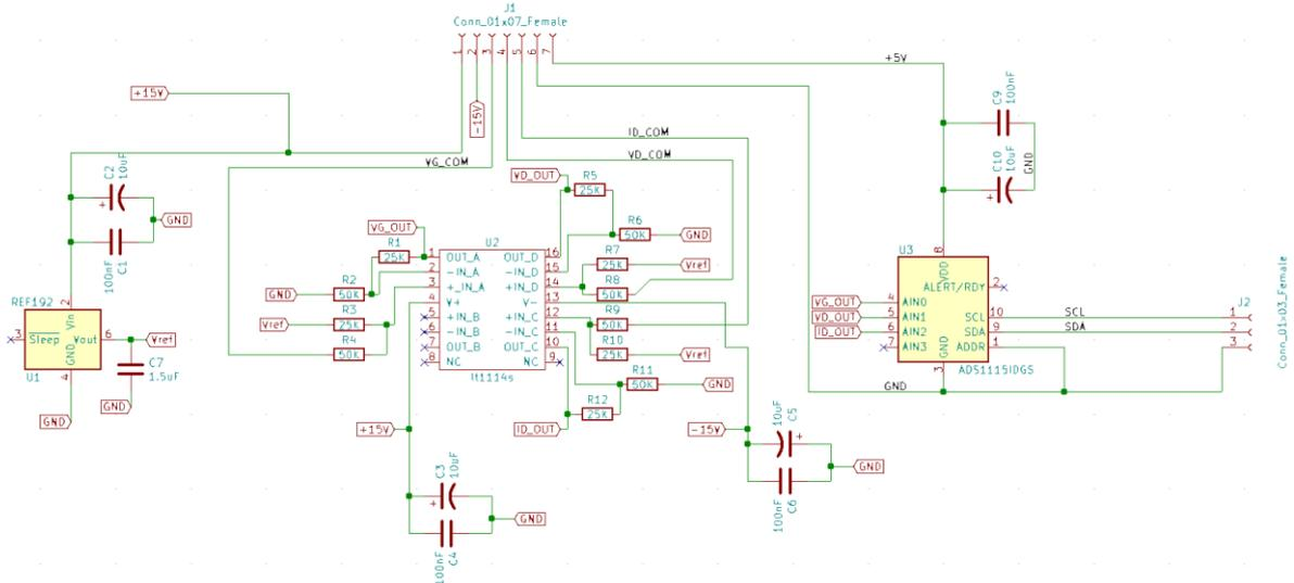
This PCB card consists of a voltage reference of 2.5V (REF192), four operational amplifiers (LT1114S) and a 16-bit ADC configured in single ended mode (ADS1115). With these three elements and the configuration of resistors, it is possible to make the change of the voltage range that was mentioned above.
