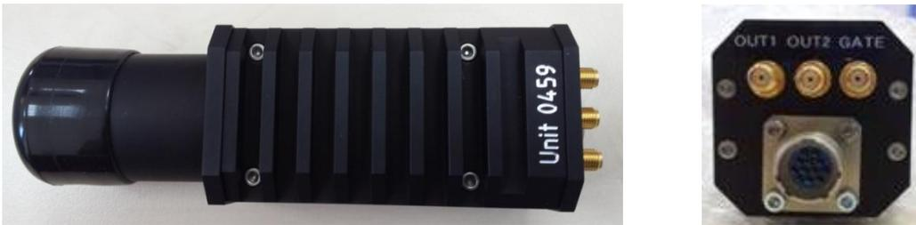
Figure 3. Detector package.
