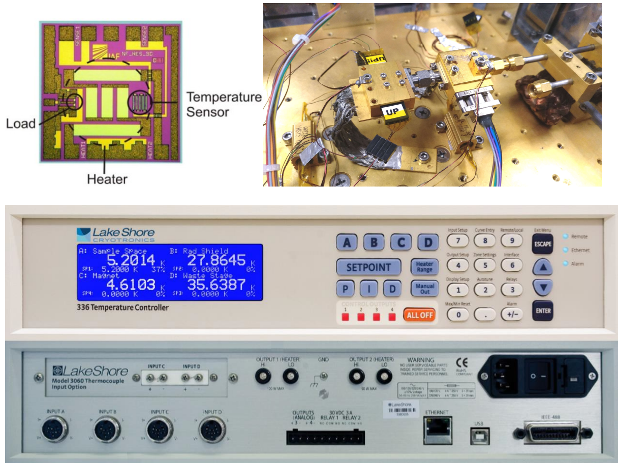
Figure 1: Up left: photo of the variable temperature cryogenic termination chip. Up right: photo of the cold plate of a cryostat with a cryogenic amplifier and a variable temperature load module connected to the input. Down: Photo of the Lake Shore 336 cryogenic temperature controller used.
