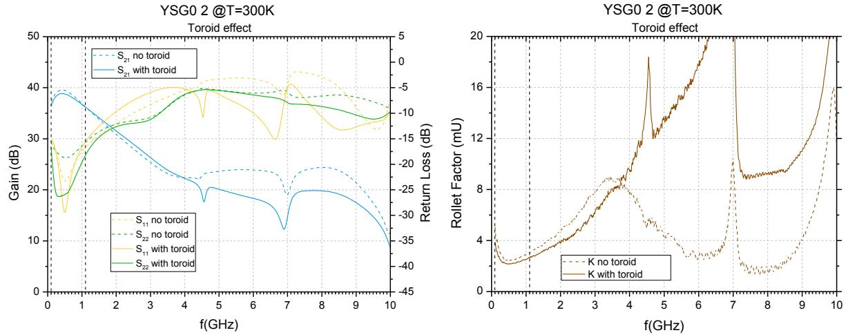
**Figure 5:** Toroid effect. Only results with the toroid and wire finally used are shown
