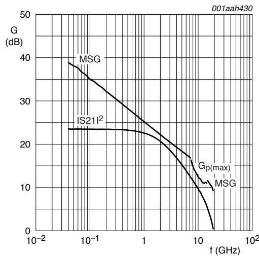
$V_{CE} = 2$  V;  $I_C = 5$  mA;  $T_{amb} = 25$  °C.
