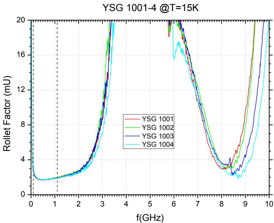
**Figure 15:** Measurement of Rollet factor of YSG amplifiers at cryogenic temperature
