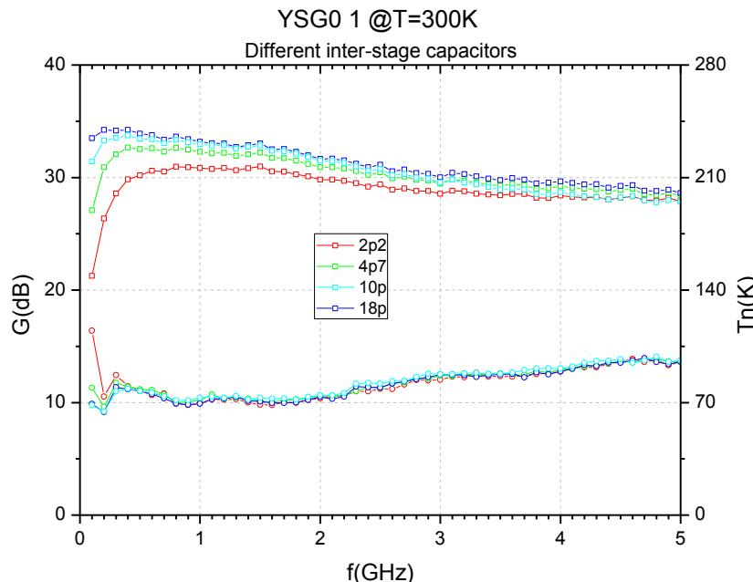
Figure 1: Noise Figure Meter measurements with different inter-stage capacitors
