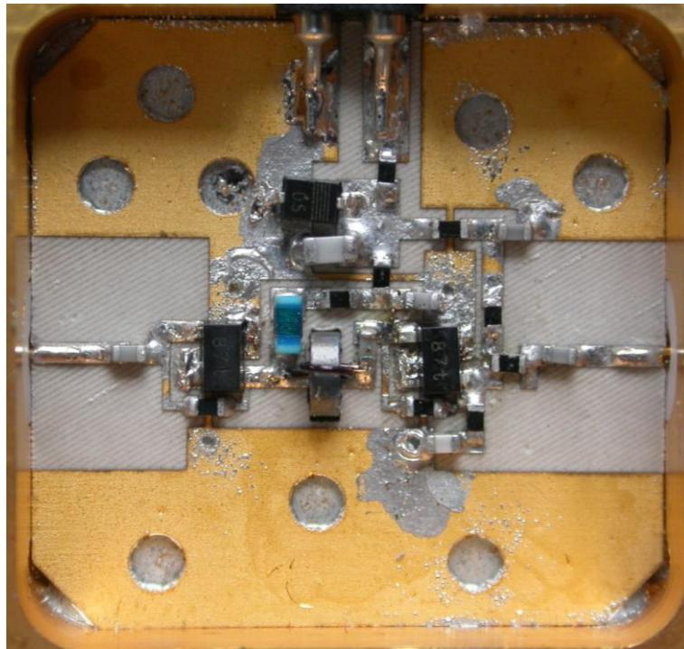
Figure 11: Internal view of YSG 1002 amplifier
