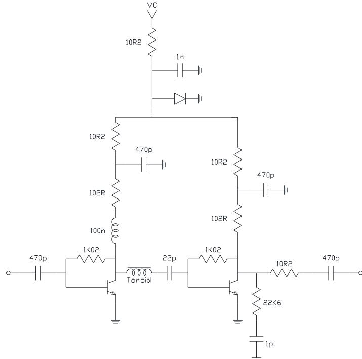
Figure 7: YSG1 amplifier final schematic
