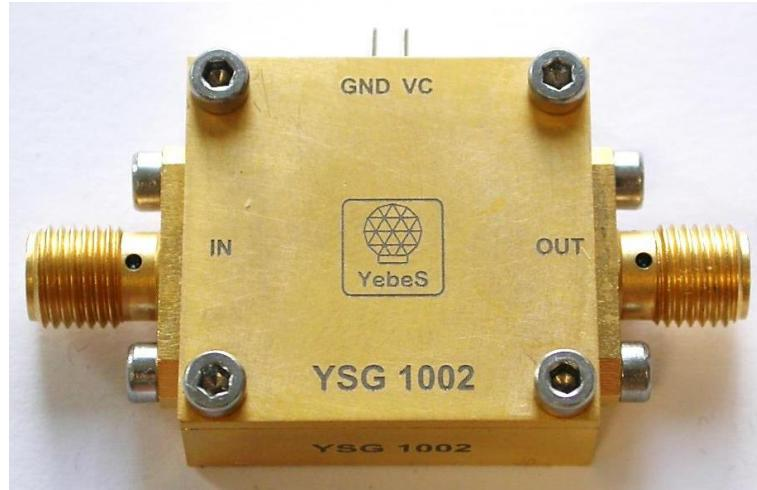
Figure 12: External view of YSG 1002 amplifier
