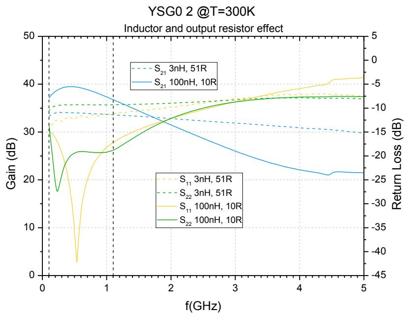
Figure 2: Inductor and output resistor effect
