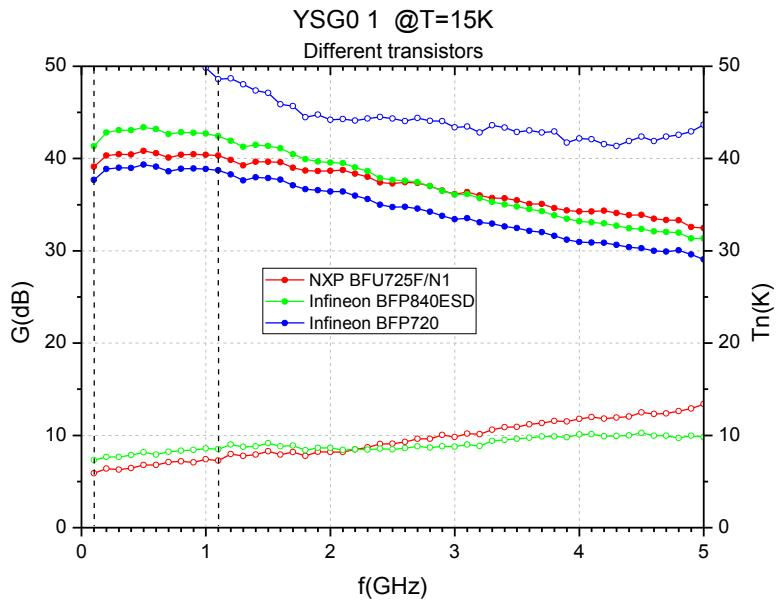
Figure 6: Transistor comparison
