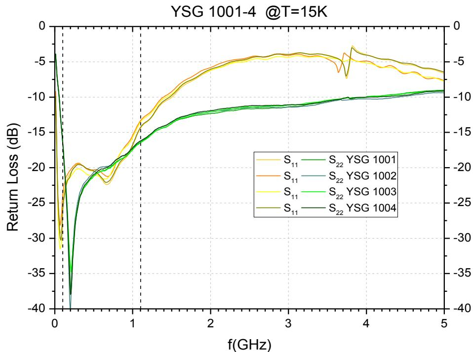
Figure 13: Measurement of return loss of YSG amplifiers at cryogenic temperature
