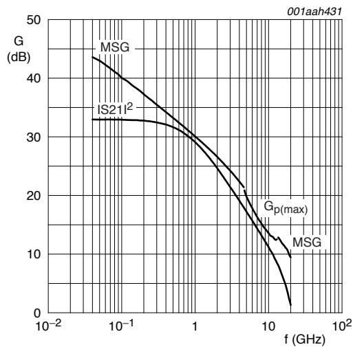
$V_{CE} = 2$  V;  $I_C = 25$  mA;  $T_{amb} = 25$  °C.
