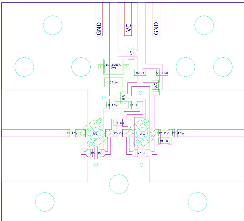
Figure 18: YSG0 amplifier substrate
