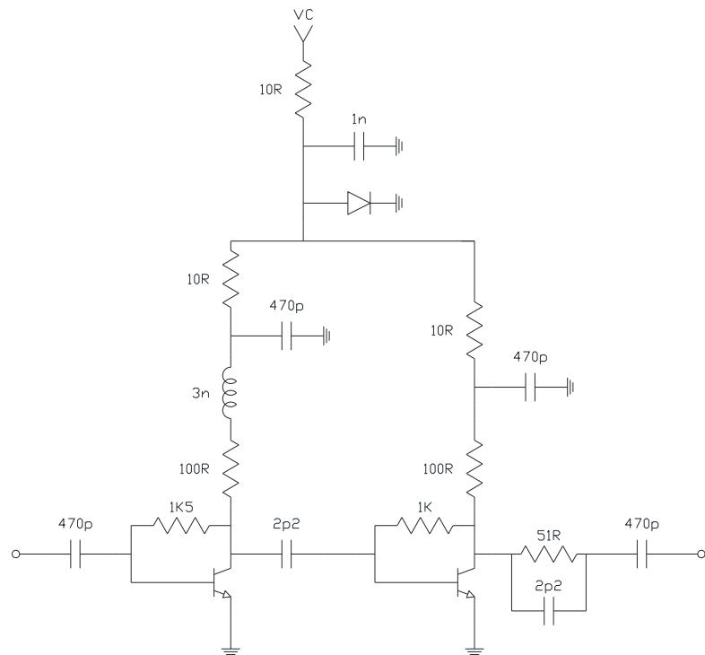
Figure 16: YSG0 amplifier schematic
