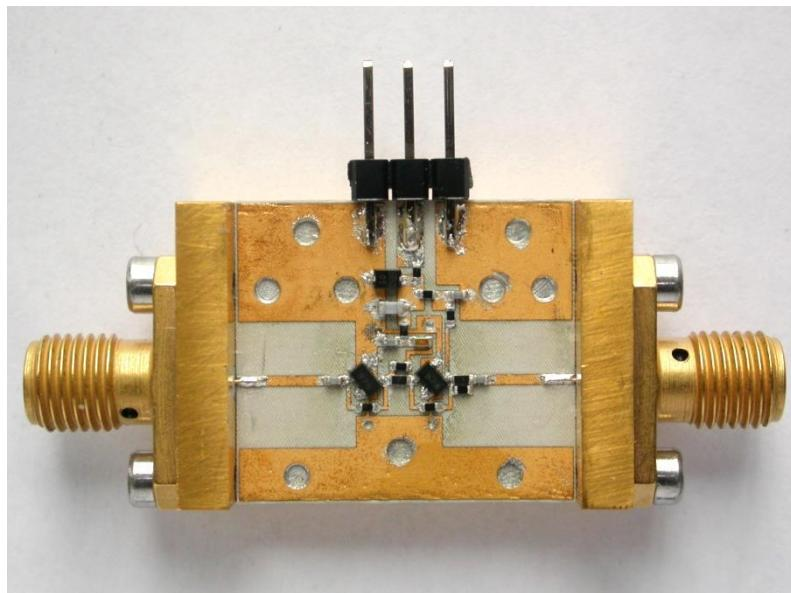
Figure 17: External view of an YSG0 LNA
