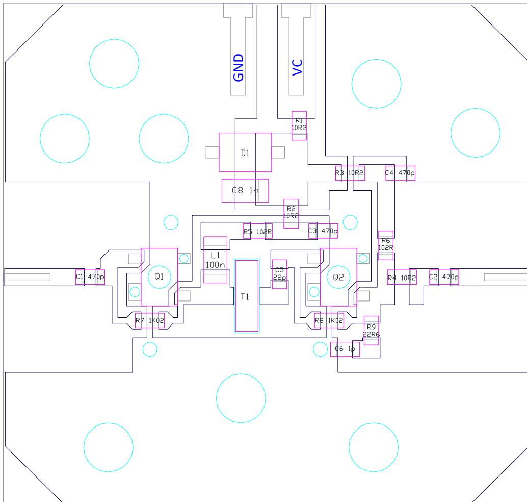
Figure 8: YSG1 amplifier substrate
