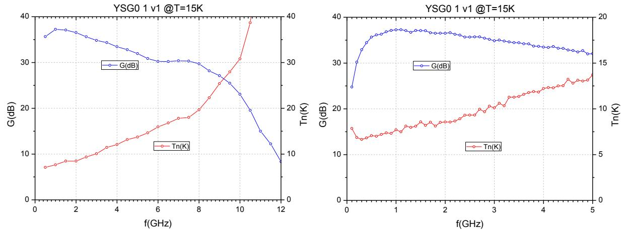
**Figure 20:** Noise and gain measurement of a YSG0 LNA at 15 K
