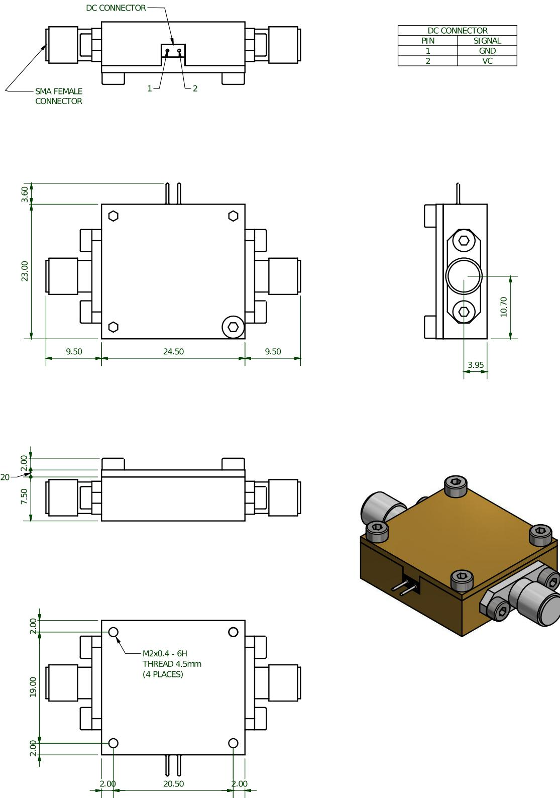
Figure 10: YSG1 mechanical and electrical interface, external dimensions and DC connector pin-out
