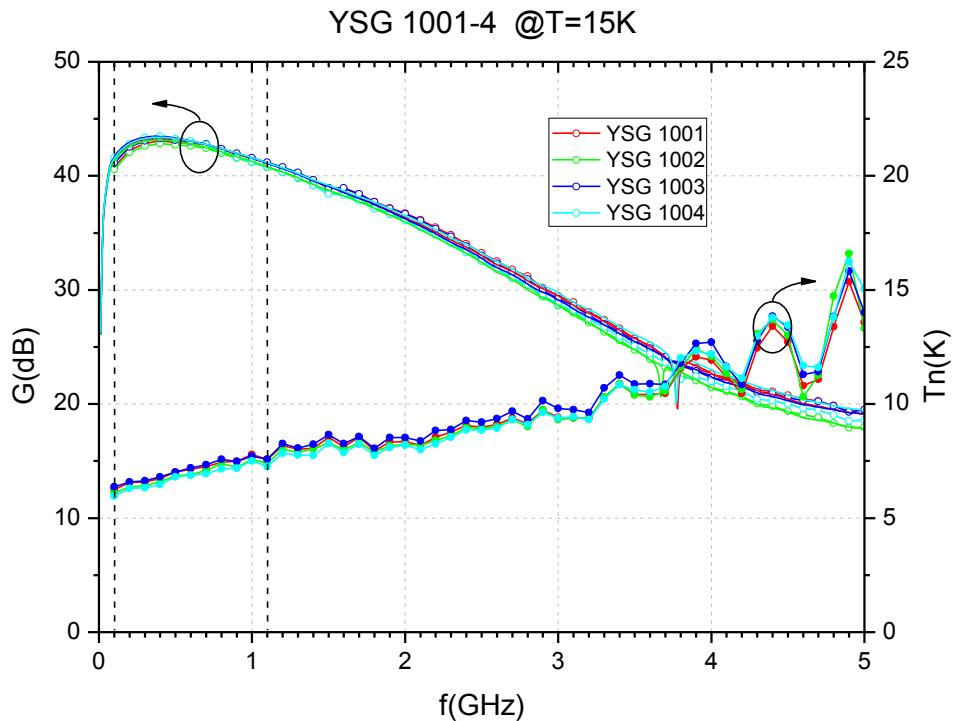
**Figure 14:** Measurement of gain and noise temperature of YSG amplifiers at cryogenic temperature
