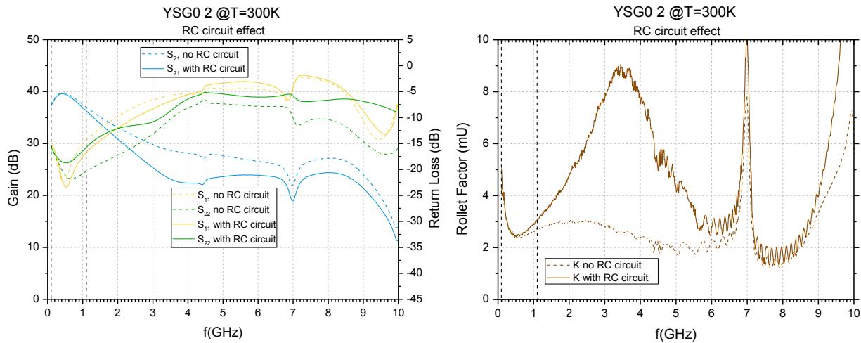
**Figure 3:** RC circuit at output effect. Note that despite the unconditional stability at room temperature, the Rollet factor always decreases upon cooling and it was lower than 1 at 8 GHz at cryogenic temperature.
