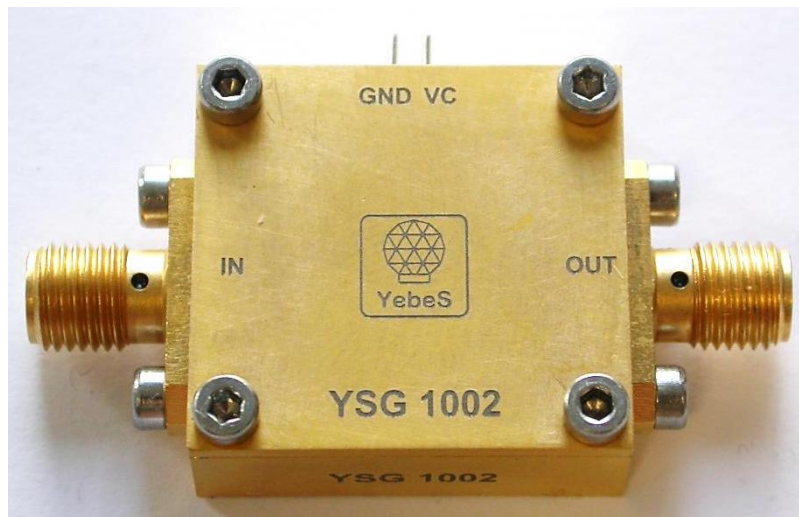
Figure 1: External view of a YSG 1 LNA. Dimensions excluding, connectors are 24.5×23×8.7 mm (X×Y×Z in the picture)
