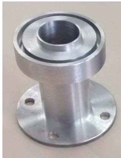
Fig. 2.3: Photograph of the new feed horn of the test channel of the holography system.
