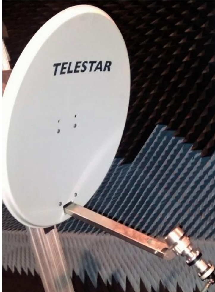
Fig. 3.4: Photograph of the new reference antenna.
