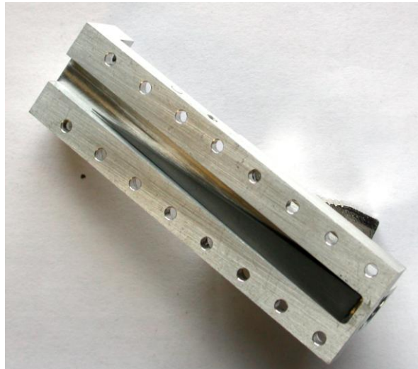
Figure 1. Wedge shaped absorber inside the WR-22 waveguide split block. This design is similar to the one used in [3].
