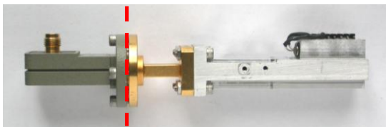
a) Measurement of the return losses of the heated load (red line in Figure 5)
