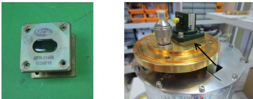
Figure 6. Vacuum window used for the vacuum tests, gain and T_{\text{noise}} measurements.
