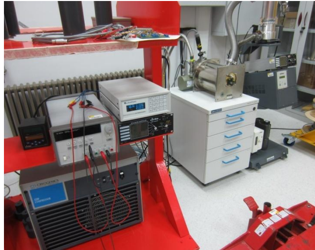
Figure 27. O'Higgins receiver, vacuum and cooling tests.
