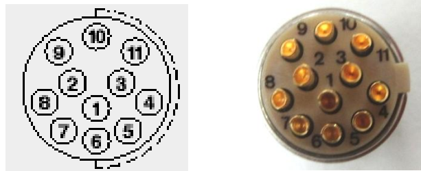
Figure 16. 11 pin Fischer ("wire" connector view (female), red point up).
