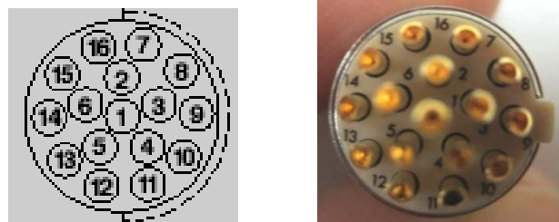
Figure 17. 16 pin Fischer ("wire" connector view (female), red point up).
