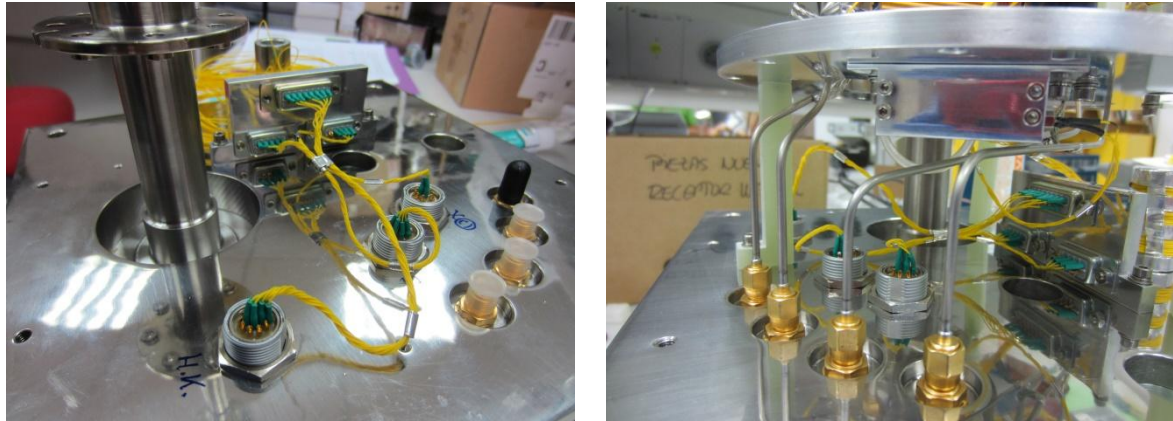
Figure 3. Dewar bottom flange, outside and inside views.
