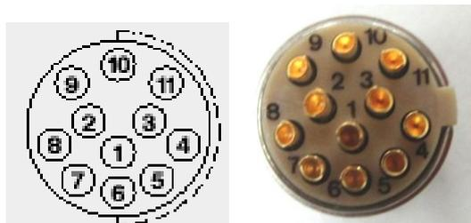
Figure 12. 11 pin Fischer ("wire" connector view (female), red point up).
