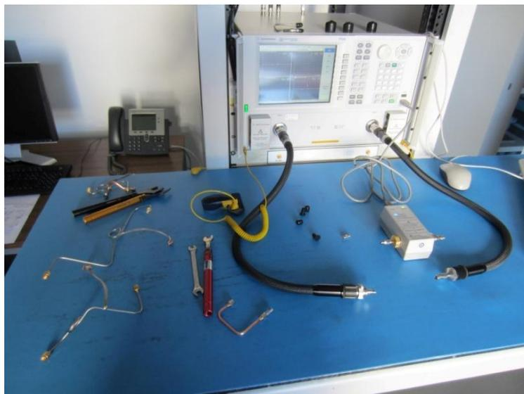
RF cables measurement setup.
