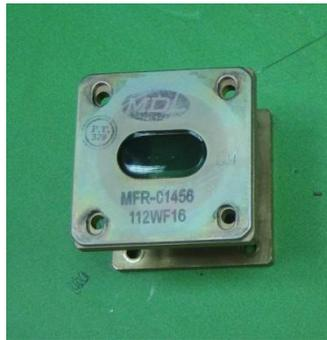
Figure 5. Vacuum window used at O'Higgins and Wettzell receivers.
