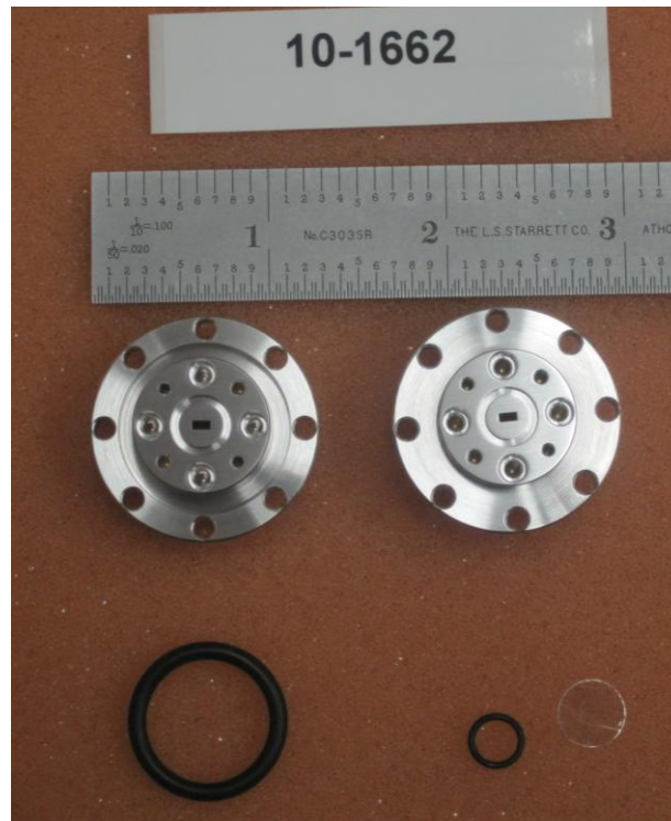
Figure 1. Hermetic WR-10 feedthrough, p/n 10-1662, from the Aerowave company.
