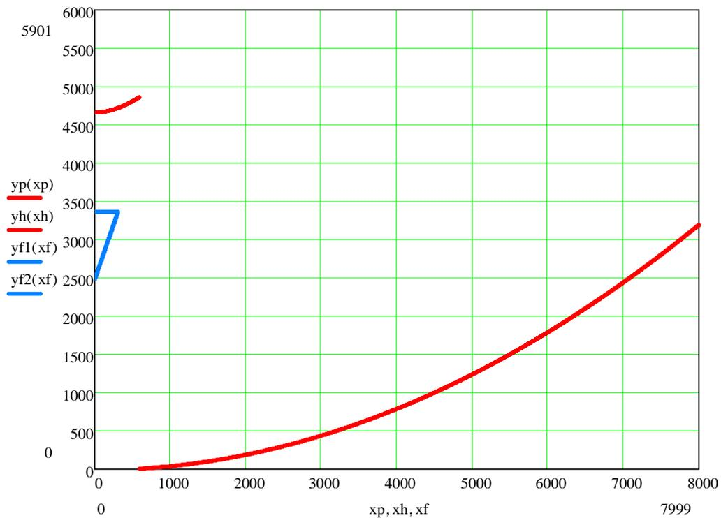
Fig. 3. One cassegrain solution geometry with feed. This geometry is used to show differences towards the alternative shape optimized cassegrain design.
