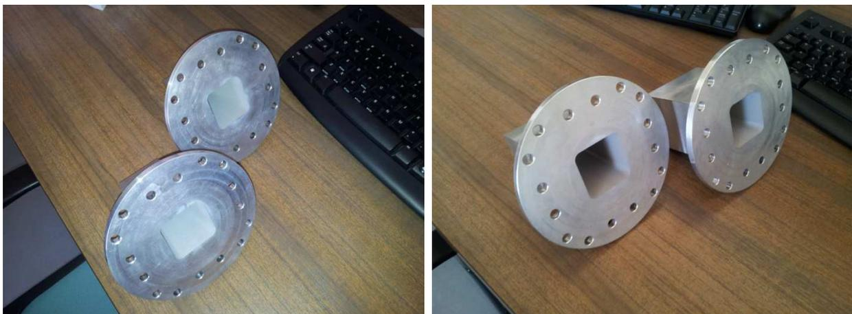
Figure 20. Two couples of WR159 and WR112 to squared waveguide transitions
