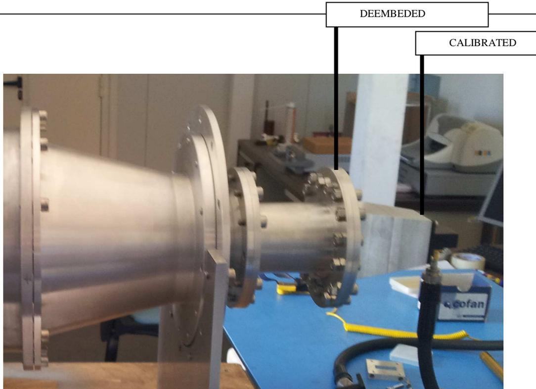
Figure 22. Measurement of port reflection setup from 4.5 GHz to 7.0 GHz. It shows the calibration plane and the deembedding transition
