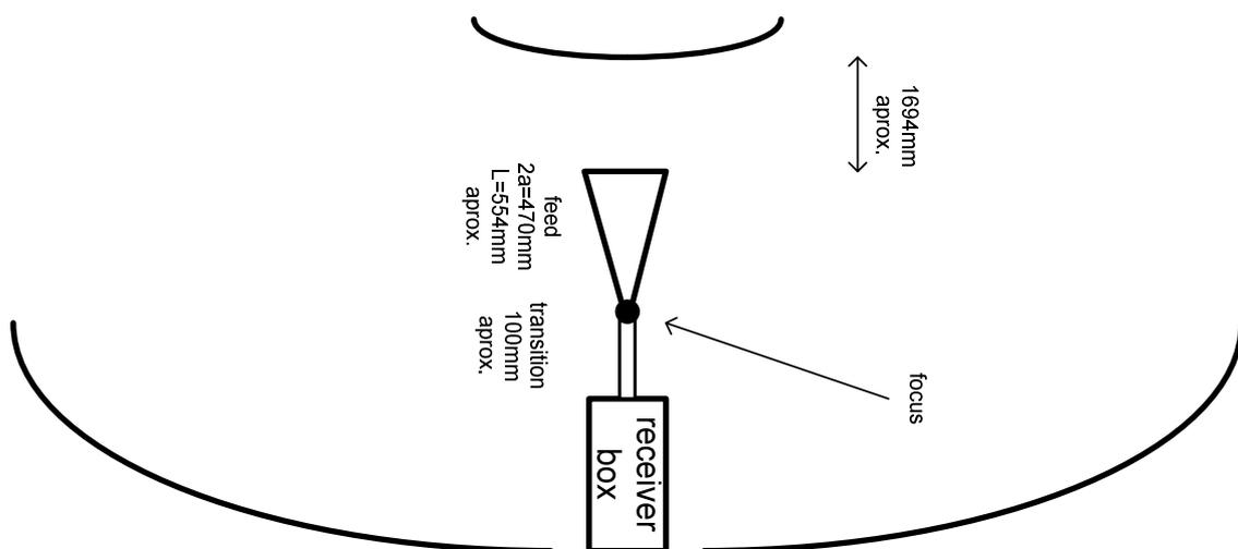
Figure 6. Layout with approximate dimensions
