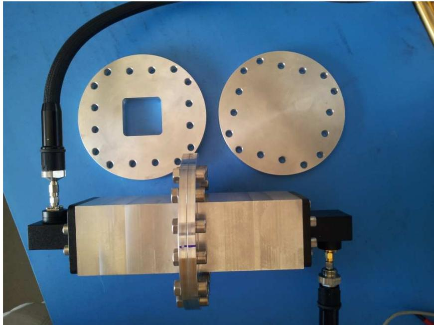
Figure 21. Thru connection for the WR159 waveguide transition. It is also shown the quarter squared waveguide and short to perform the TRL calibration
