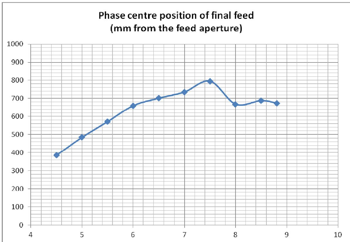
Figure 25. Feed phase centre measured from the feed aperture
