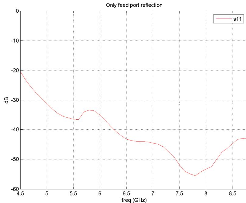
Figure 2. Feed port reflection in circular waveguide
