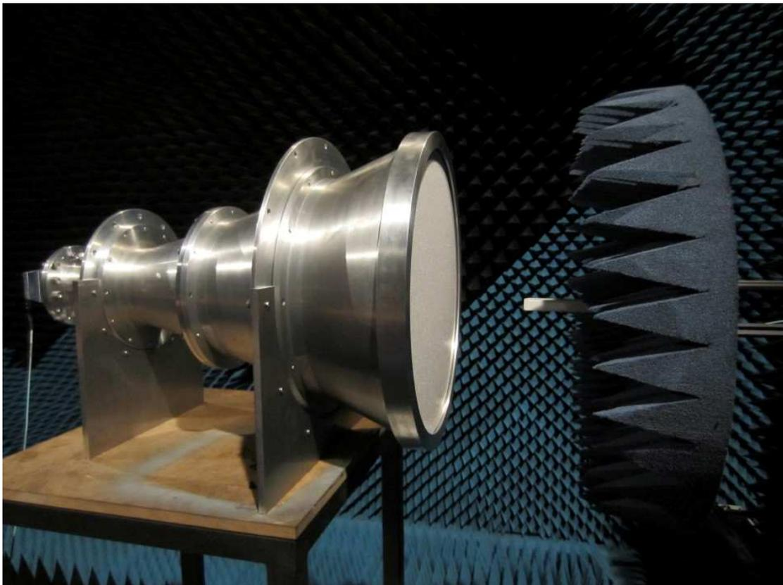
Figure 24. Measurement of radiation pattern in anechoic chamber
