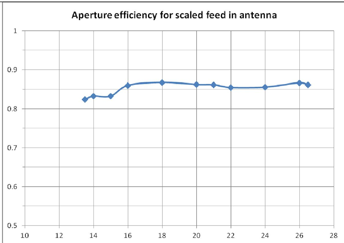
Figure 18. Aperture efficiency using the measured data of scaled feed standing in a fixed position in the antenna.
