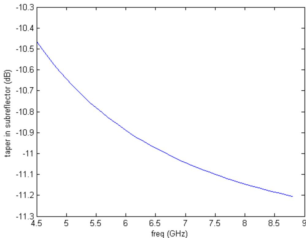
Fig. 1. Taper of feed in subreflector.
