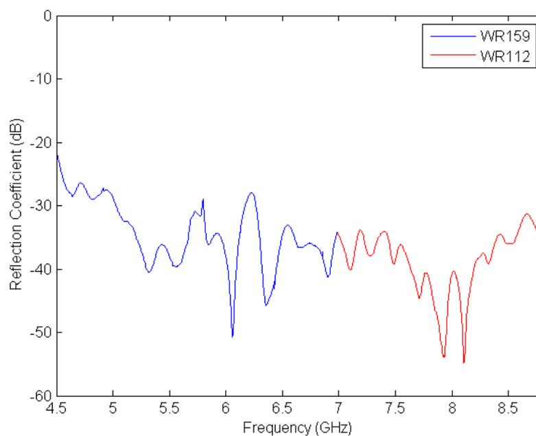
Figure 23. Measurement port reflection from 4.5 GHz to 8.8 GHz. Combination of both measurements after calibration and deembedding.
