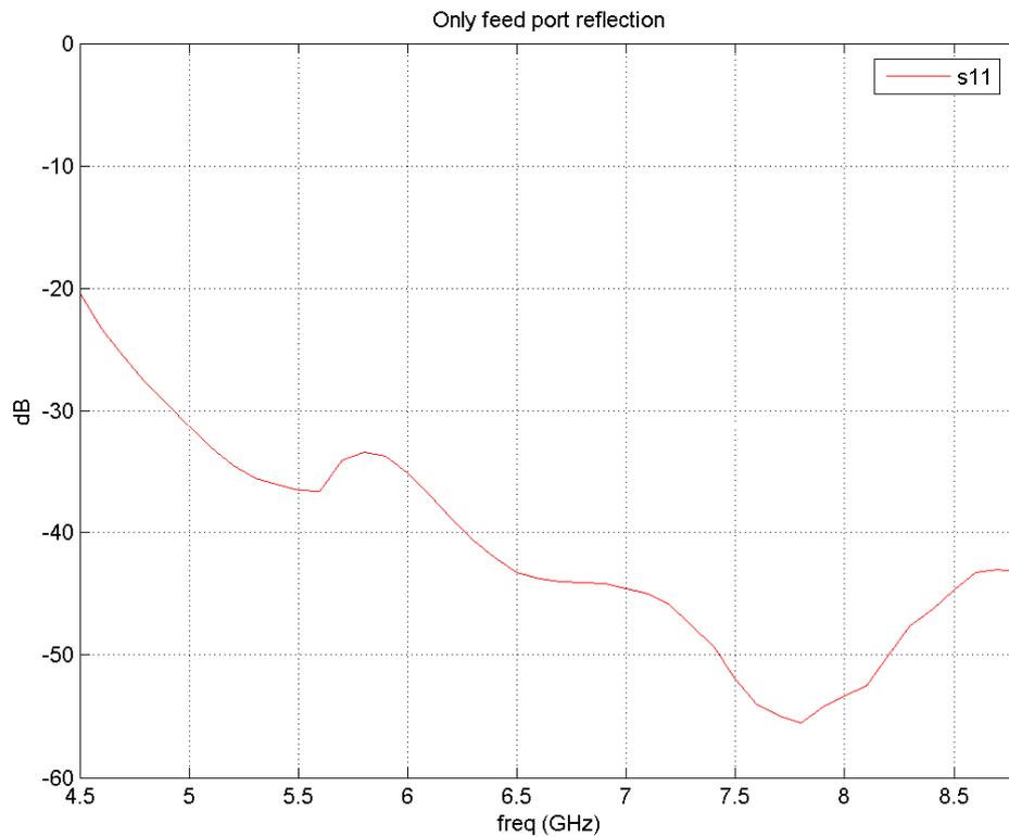
Figure 8. Feed port reflection in circular waveguide
