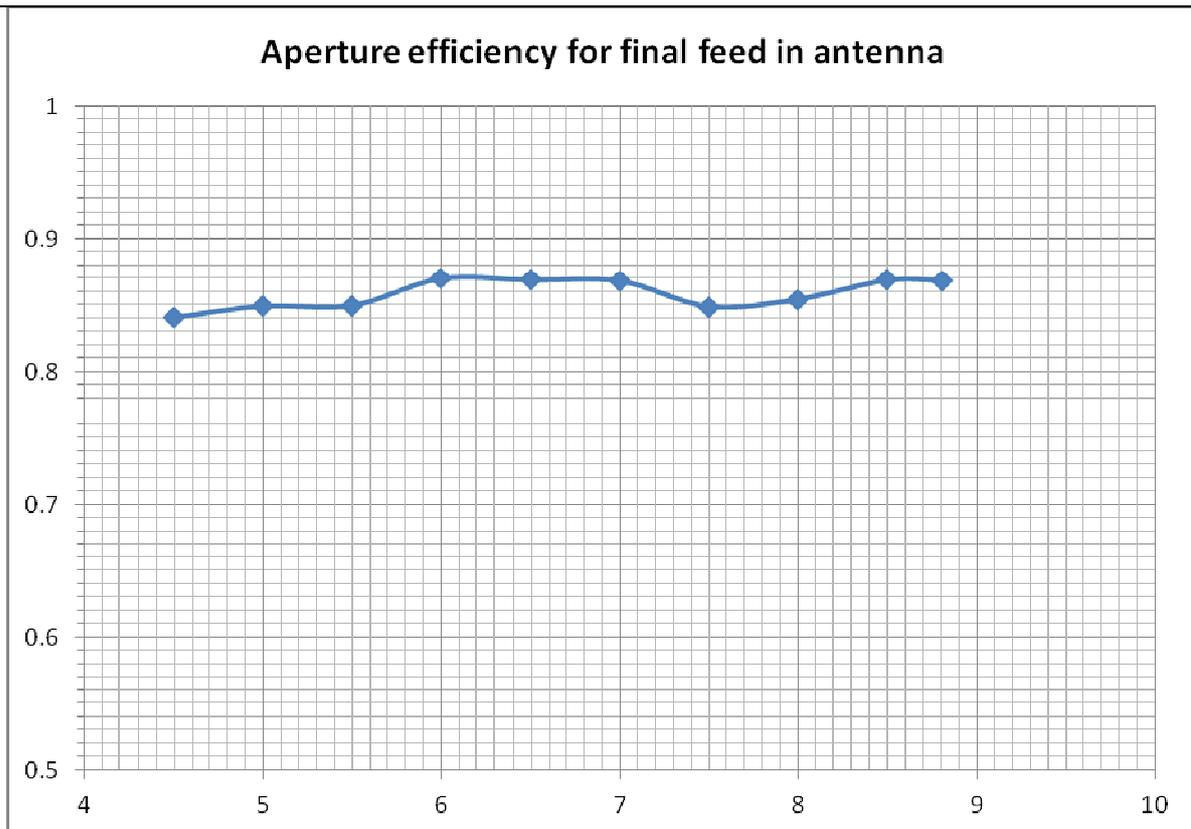
Figure 26. Aperture efficiency using the measured data of final feed standing in a fixed position in the antenna. The focal point of the antenna is at 660mm from the feed aperture.
