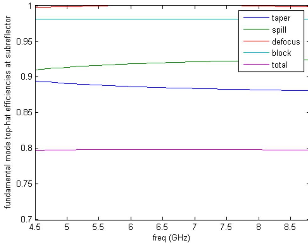
Fig. 2. Aperture efficiency over the bandwidth
