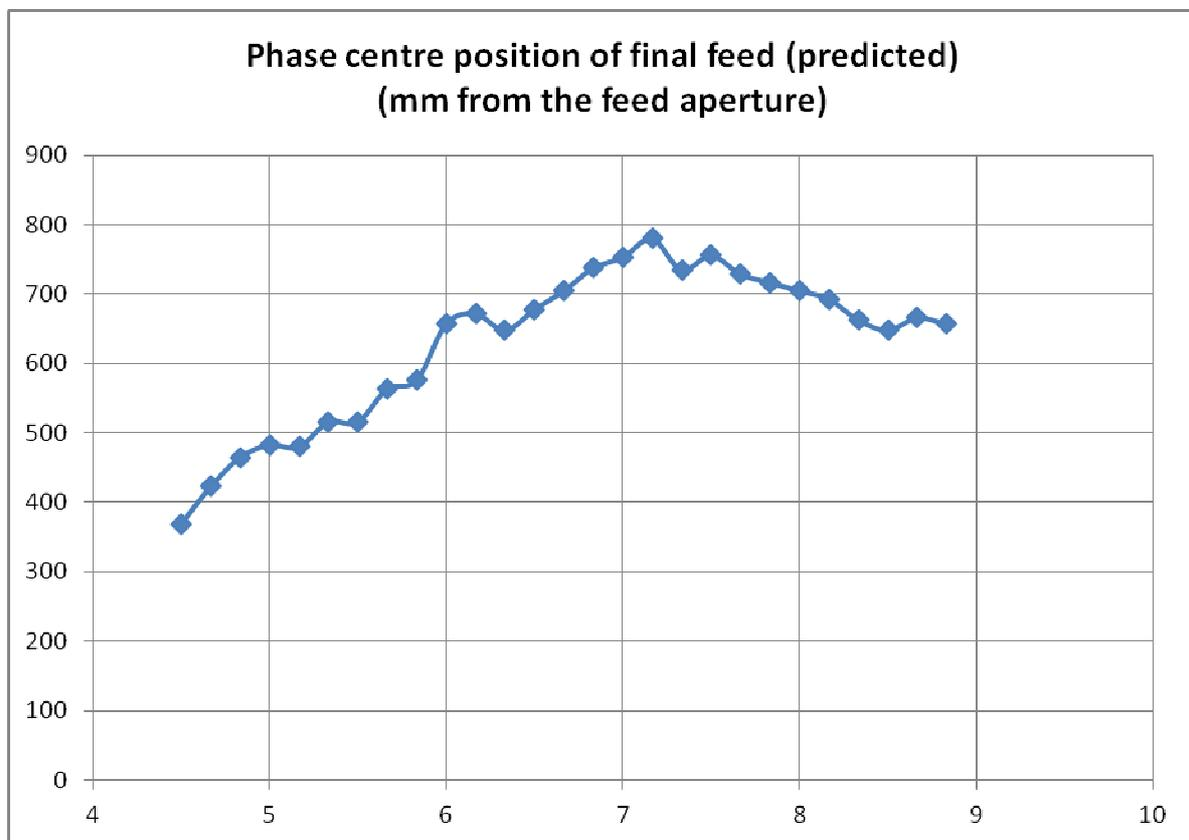
Figure 19. Prediction of the phase centre of the final feed
