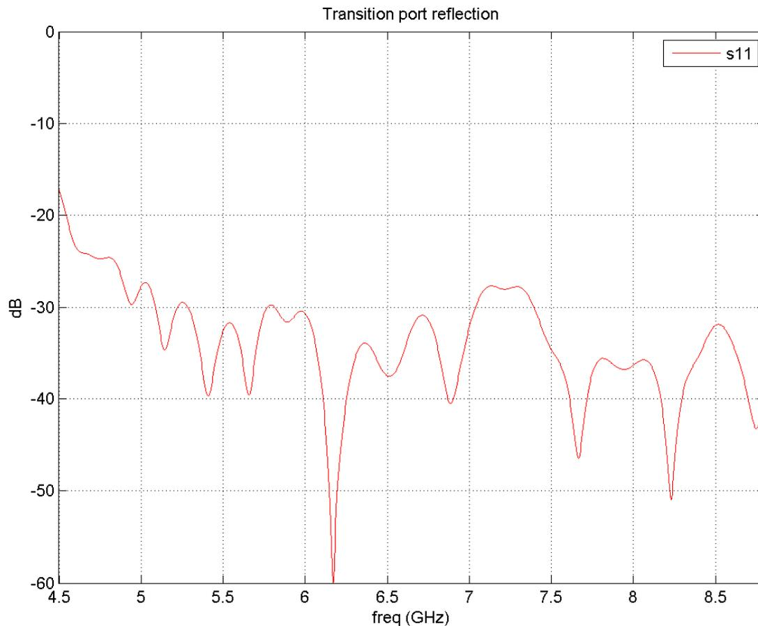
Figure 14. Feed and transition reflection
