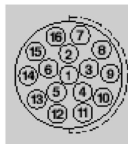
Figure 7: 16 pin Fischer (connector view, red point up).
