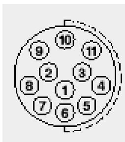
Figure 6: 11 pin Fischer (connector view, red point up).
