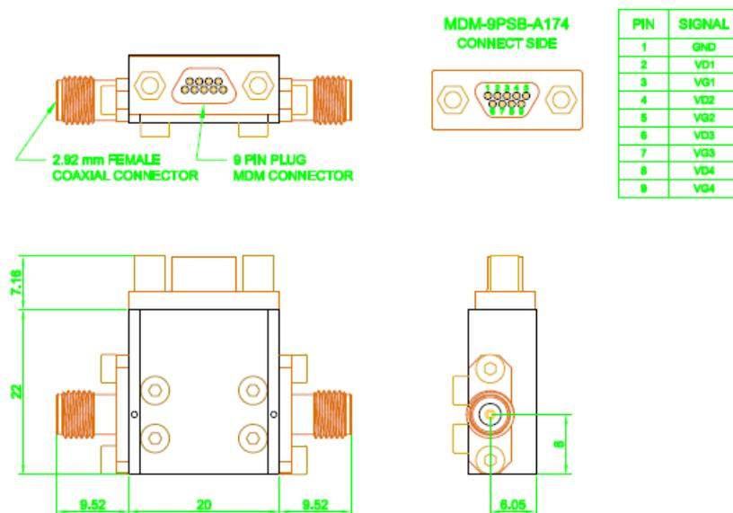
Figure 8. LNAs biasing pin-out.
