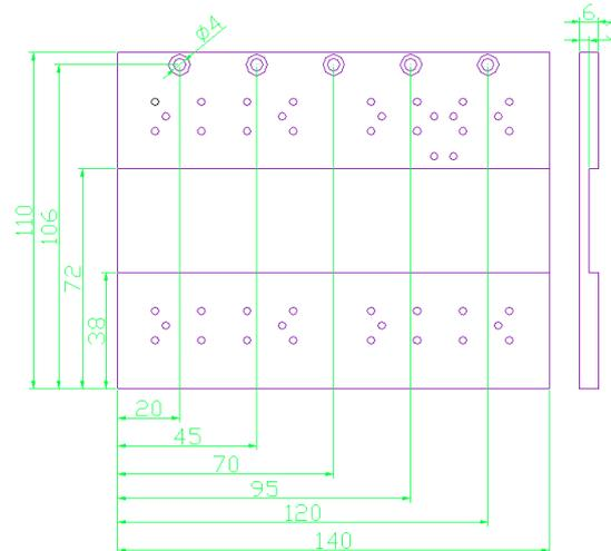
Figure 5. Cold stage plate designed for LNAs integration.
