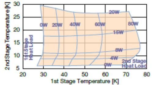
Figure 10. Typical refrigeration capacity of the model SRDK-408S2 cryocooler (50 Hz).
