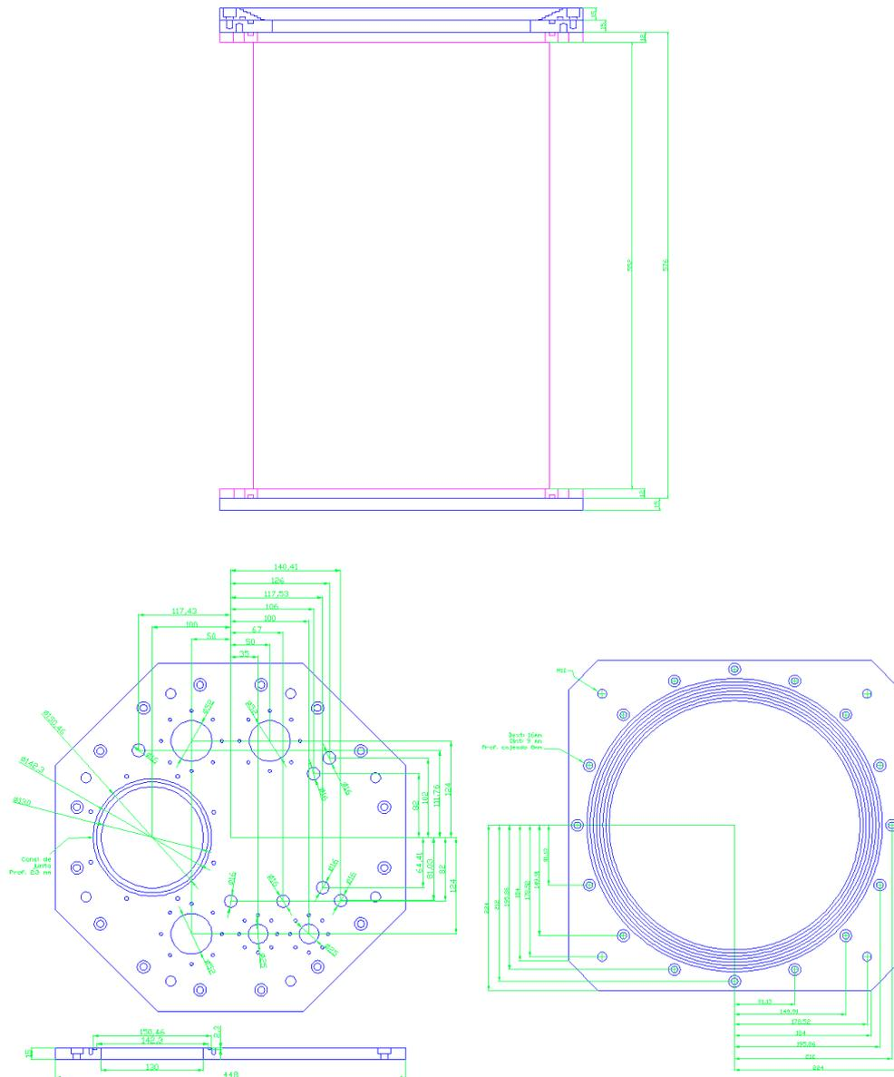
Figure 2. Dewar design: cylinder, bottom and top covers.
