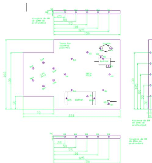
Figure 4. Cold Cu plate design
