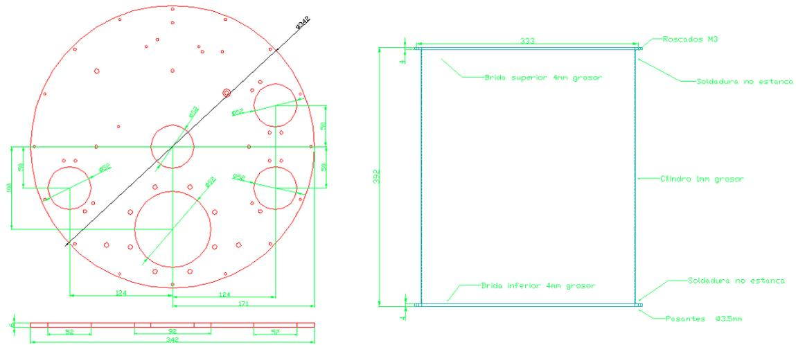
Figure 3. Intermediate stage design and radiation shield.
