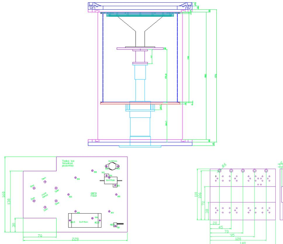
Figure 1. Cryostat overview: cold head (light blue), vacuum case (pink and dark blue), radiation shield (blue), intermediate stage (red) and cold stage (violet).
