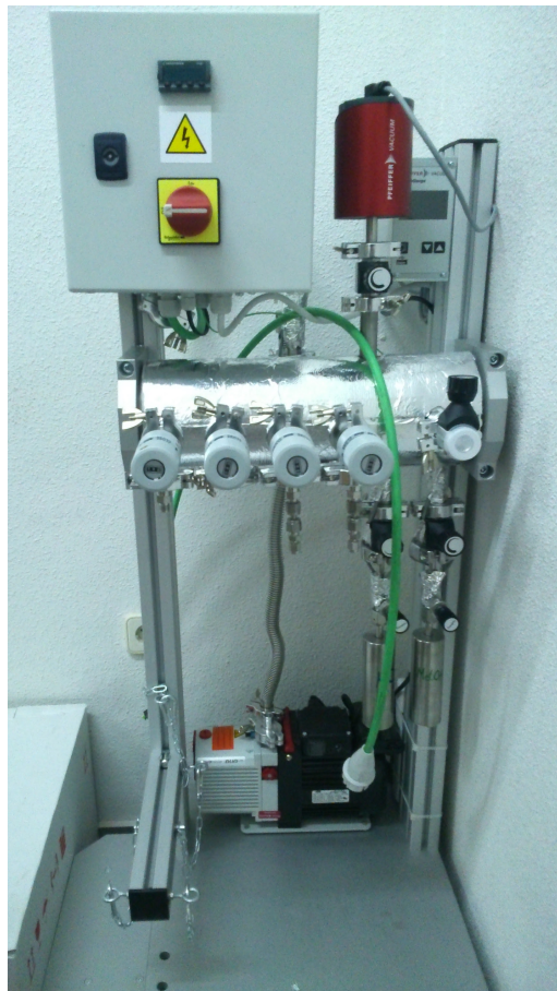
Figure 2: Gas cell: mixing chamber
