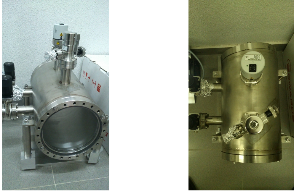
Figure 3: Gas cell with Quartz windows. Left panel: front view. Right panel: upper view.
