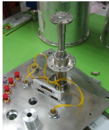
Figure 15: LNAs biasing connectors and housekeeping connector.
