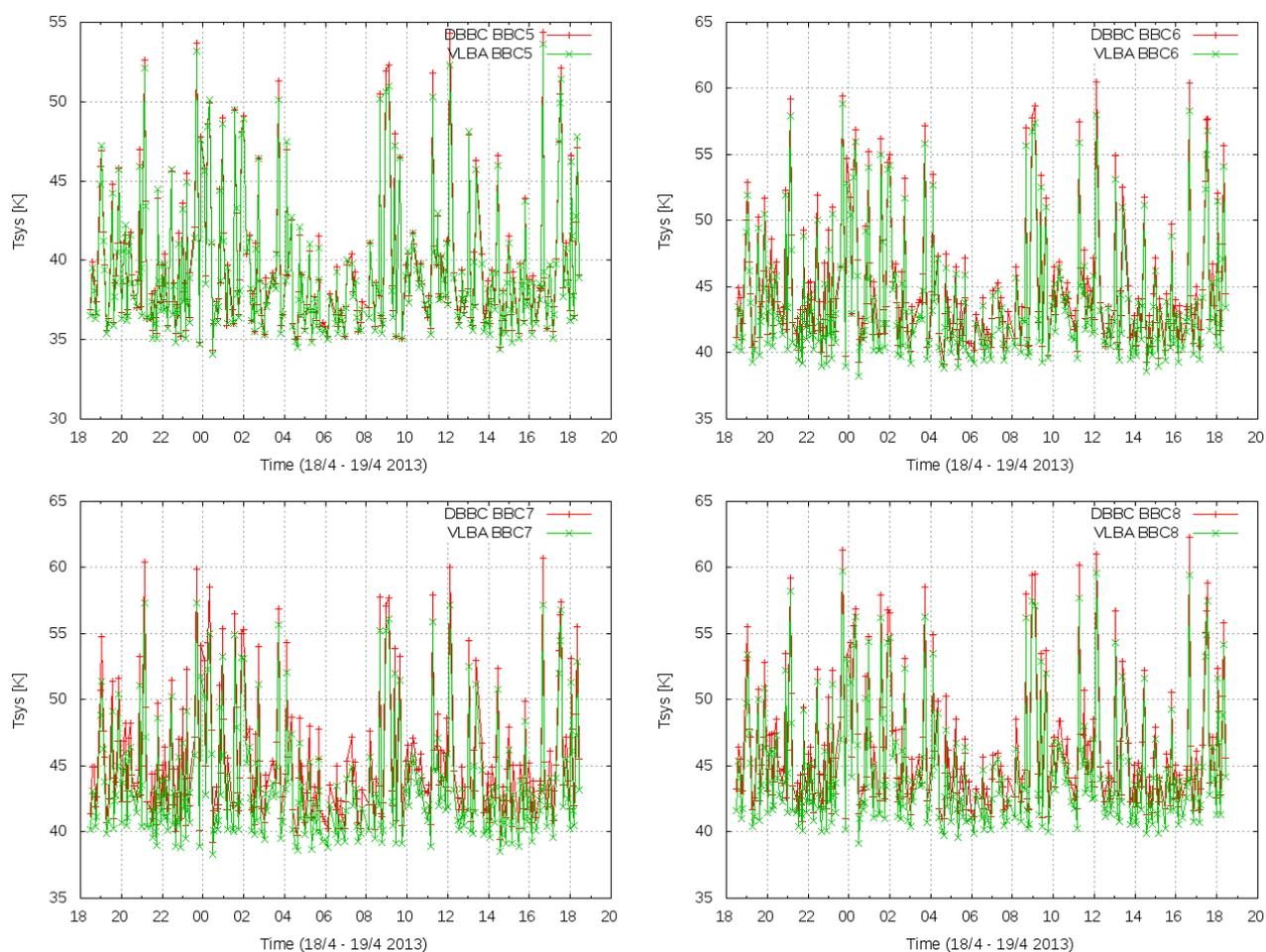
Figure 12: System temperature for IVS R4581 using the VLBA terminal and the DBBC in DDC mode (version 102) for BBCs 5 to 8.
