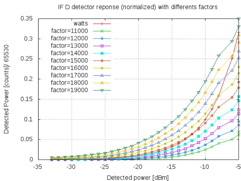
Figure 22: Normalized detected power versus detected power in dBm using a spectrum analyzer. IF D
