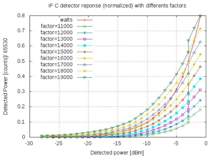
Figure 21: Normalized detected power versus detected power in dBm using a spectrum analyzer. IF C
