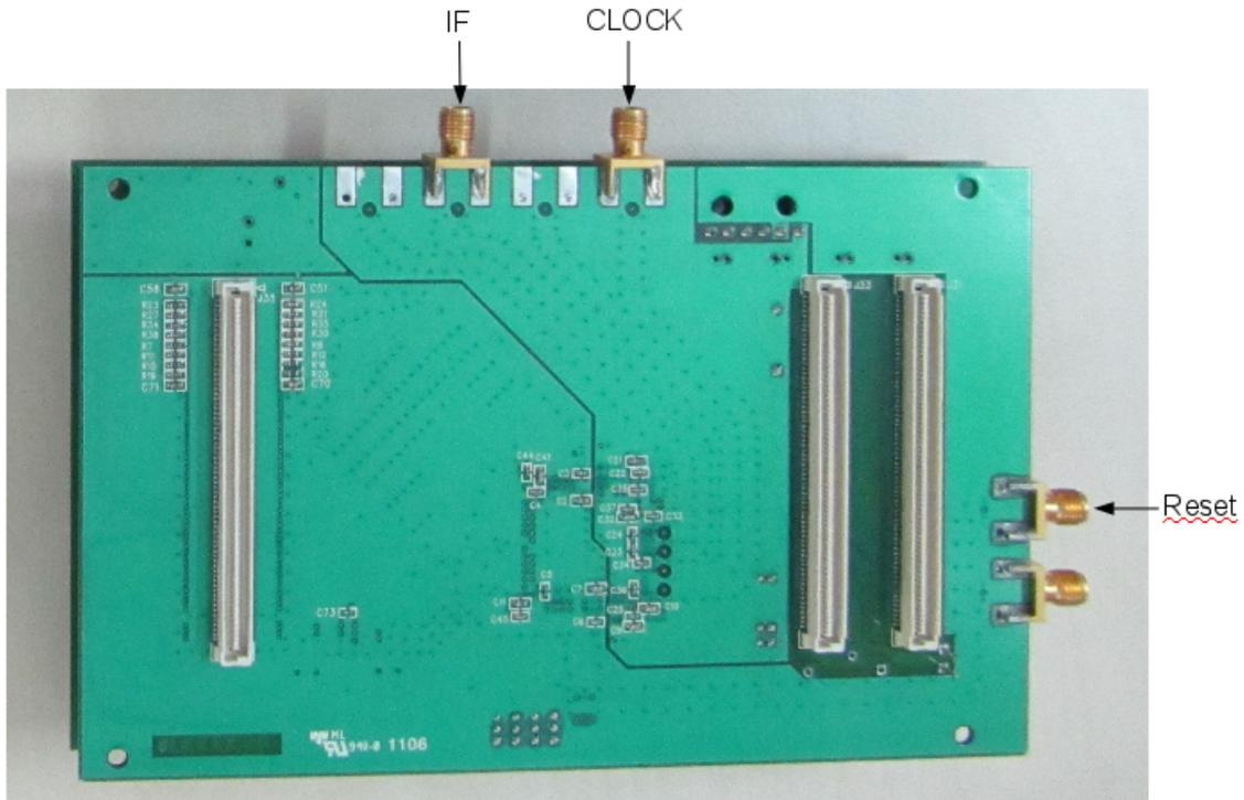
Figure 4: ADB1 board with input connectors annotated
