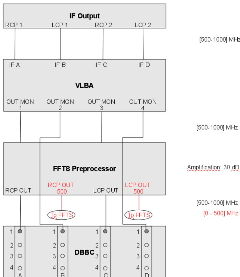
Figure 1: Current IF - DBBC setup
