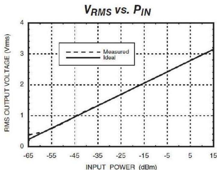
Figure 3: Voltage power detected by circuit HMC610LP4 in the band as a function of the input power
