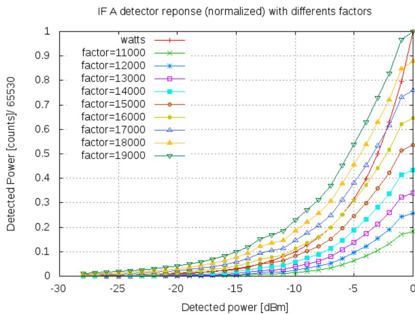
Figure 19: Normalized detected power versus detected power in dBm using a spectrum analyzer. IF A
