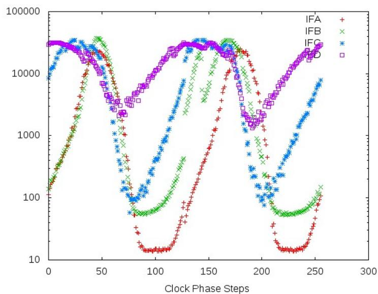
Figure 5: Results from phase calibration. The optimum value for each IF was chosen for the minimum value. Since the dynamic range is quite large a logarithmic scale was used. The chosen values were 94, 89, 79 and 192 for IFs A, B, C and D respectively.
