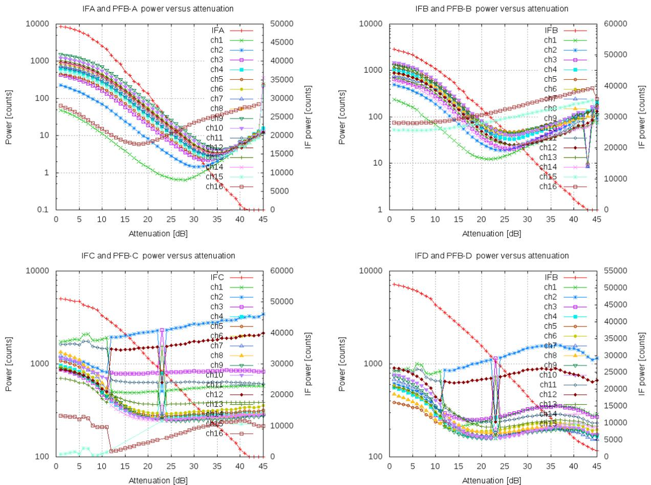
Figure 8: Power detection in the four IFS and PFB channels. The scale is linear in all cases.
