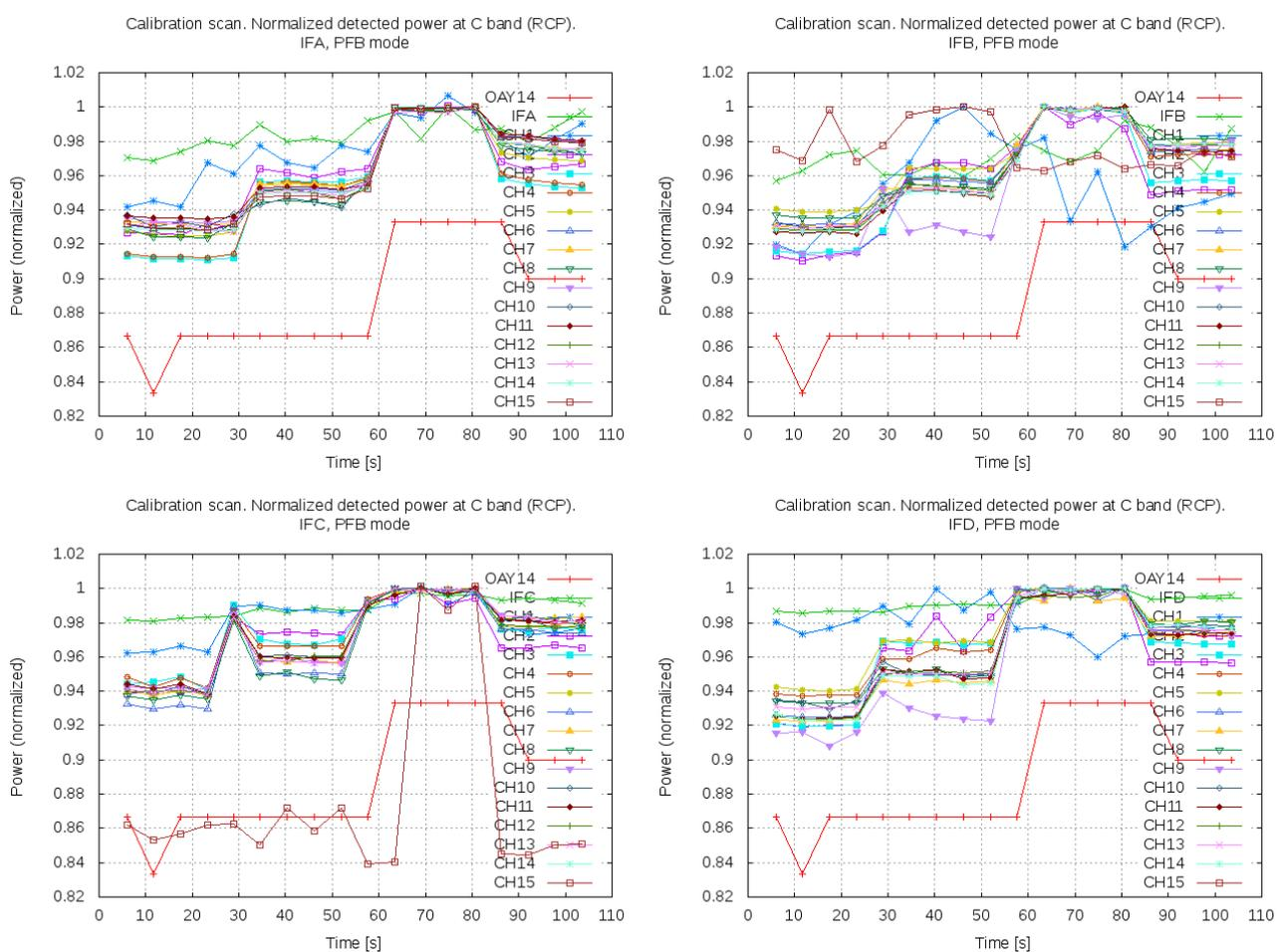
Figure 17: Calibration scan, PFB mode. Normalized detected power versus time. IF was set to a manual level of 38000 counts and individual channels were set to manual. Panels, upper left: RCP, IFA, lower left: LCP, IFB, upper right: RCP, IFC, lower right: LCP, IFD. The last subscan was suppressed
