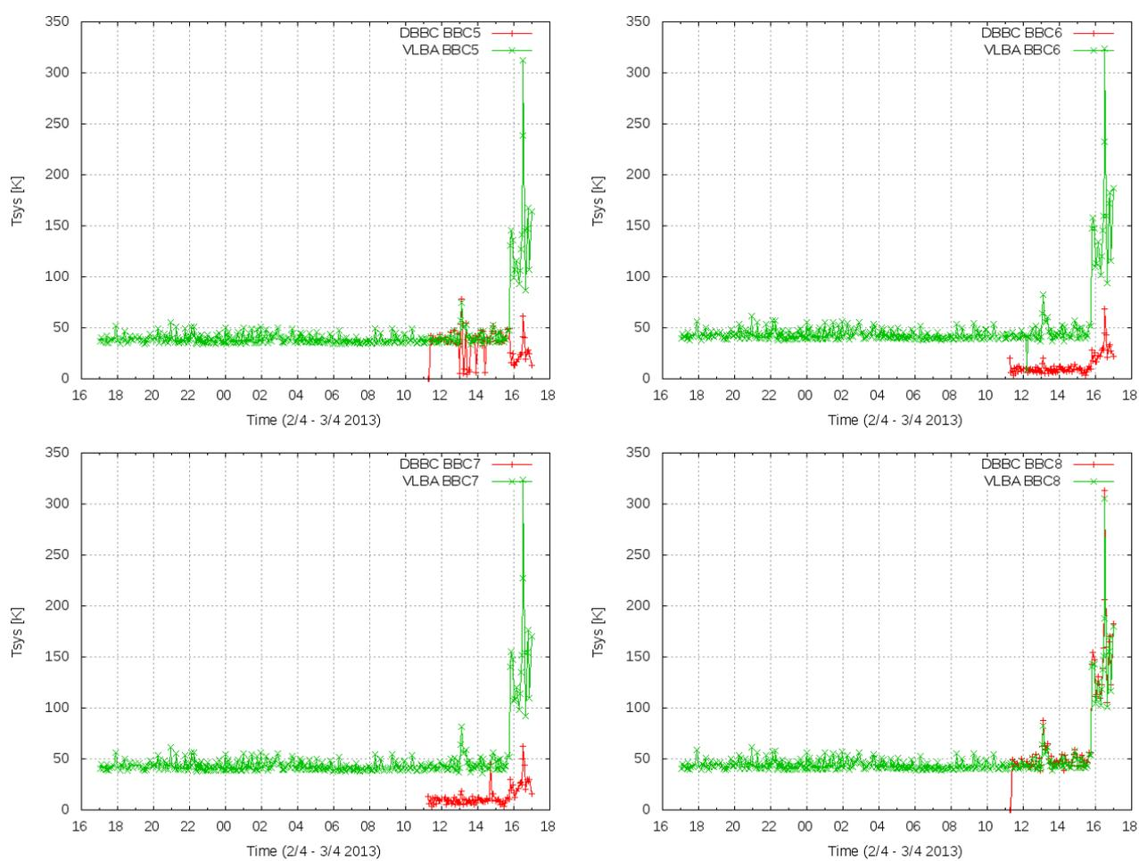
Figure 10: System temperature for IVS R1579 using the VLBA terminal and the DBBC in DDC mode (firmware version 103) for BBCs 5 to 8.
