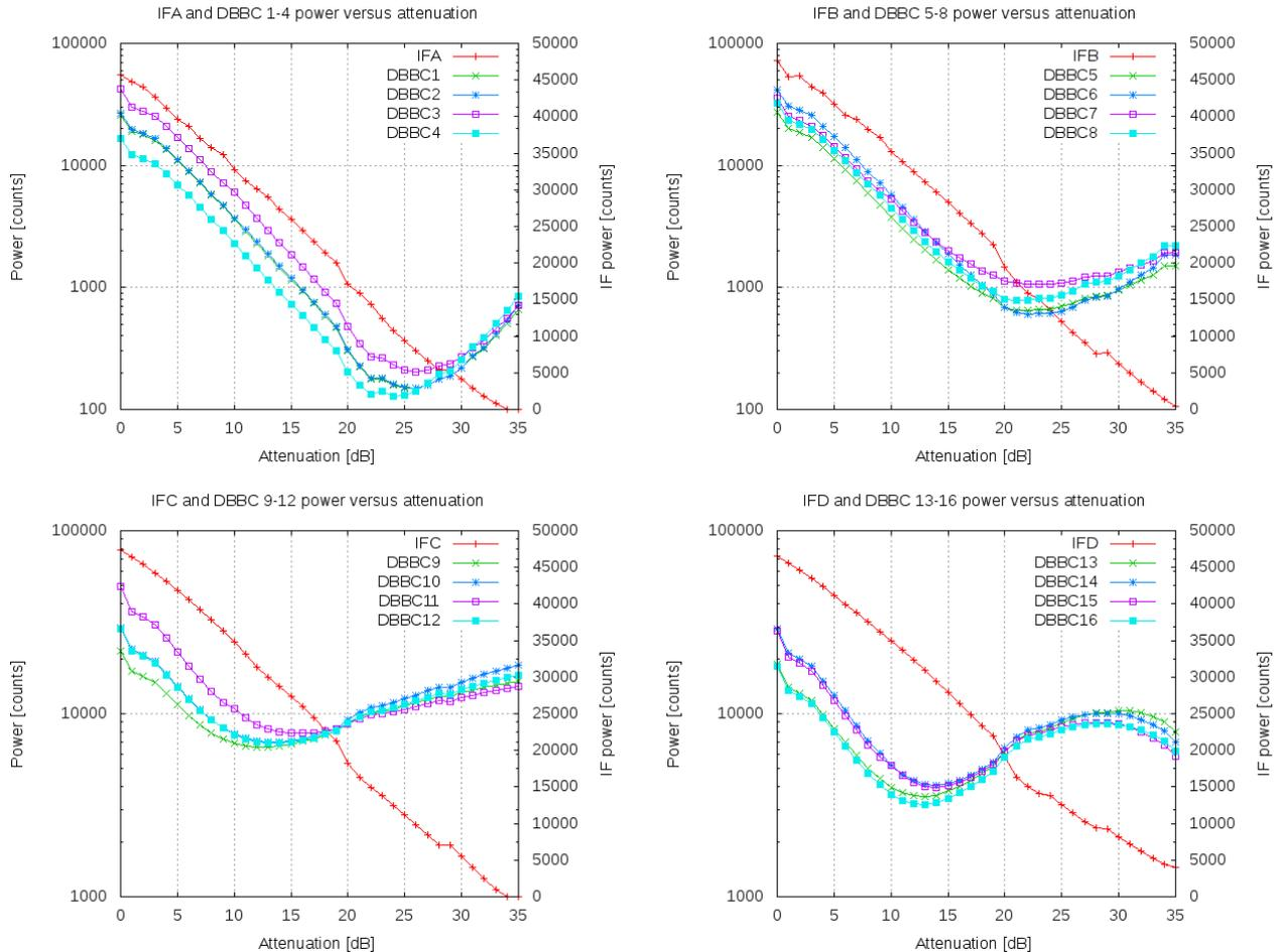
Figure 7: Power detection in the four IFs and BBC channels 1 to 16. The scale is logarithmic (left y axis) for individual channels and linear (right y axis) for the IF power counts. The dual scale mode allows to compare the regime at which all detectors work linearly
