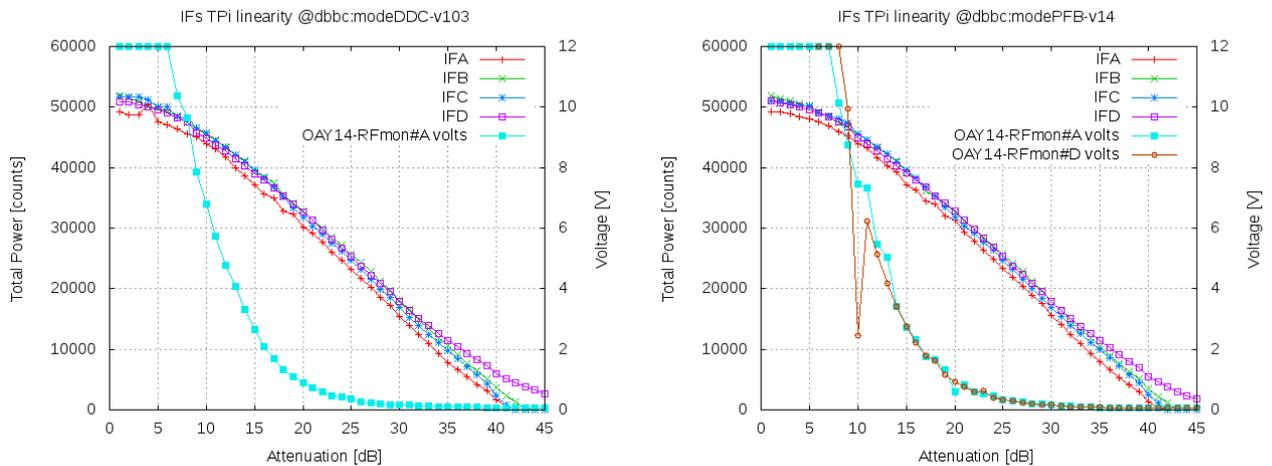
Figure 6: Power detection in arbitrary units and voltage as a function of input power. Left panel: DDC mode (firmware v103). Right panel: PFB mode (firmware v14)
