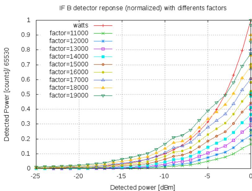
Figure 20: Normalized detected power versus detected power in dBm using a spectrum analyzer. IF B
