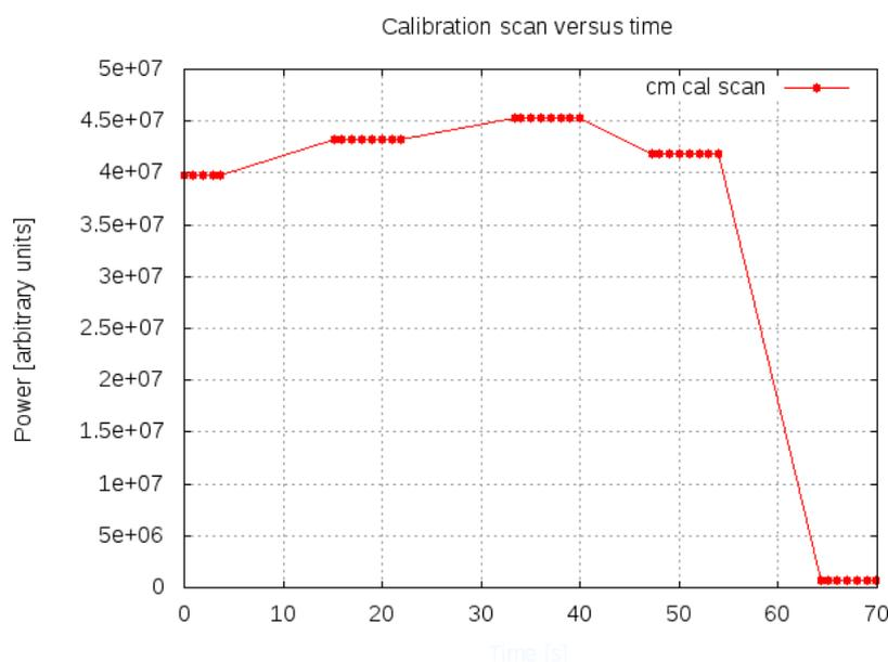
Figure 13: Typical *cm* calibration scan with 5 subscans: *Off-caloff*, *Off-calon*, *On-caloff*, *On-calon*, *zero*
