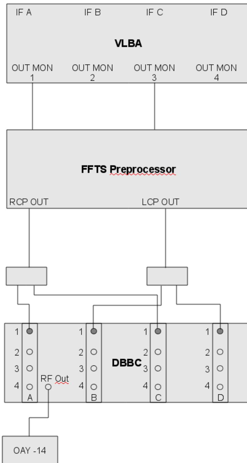
Figure 14: Setup used to do the calibration scans. The power was measured simultaneously at IFS A and C and B and D. The detected power was also monitored with continuum detector OAY-14 connected to IFA.
