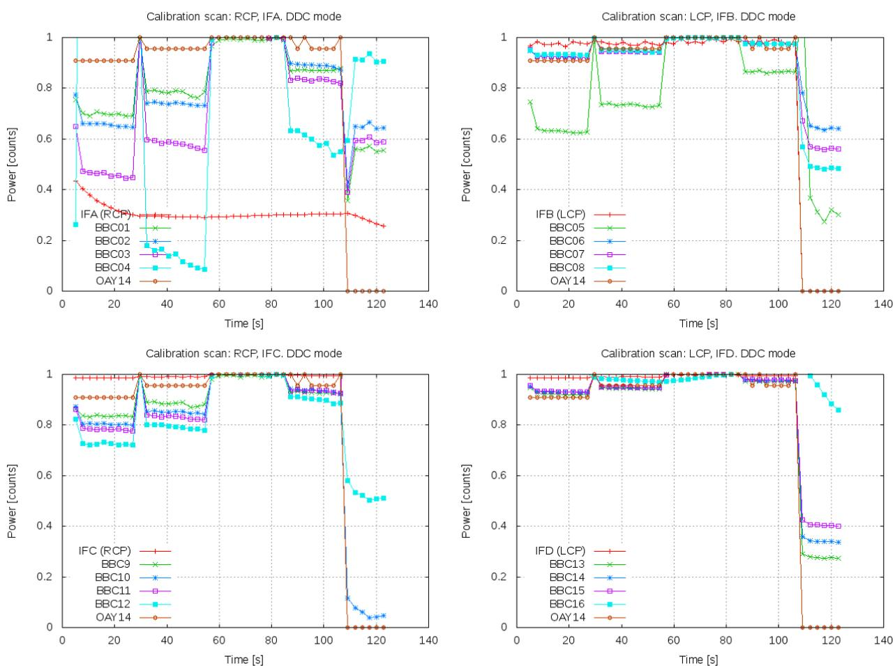
Figure 15: Calibration scan, DDC mode. Normalized detected power versus time. IF was set to a manual level of 38000 counts and individual channels were set to manual. Panels, upper left: RCP, IFA, lower left: LCP, IFB, upper right: RCP, IFC, lower right: LCP, IFD
