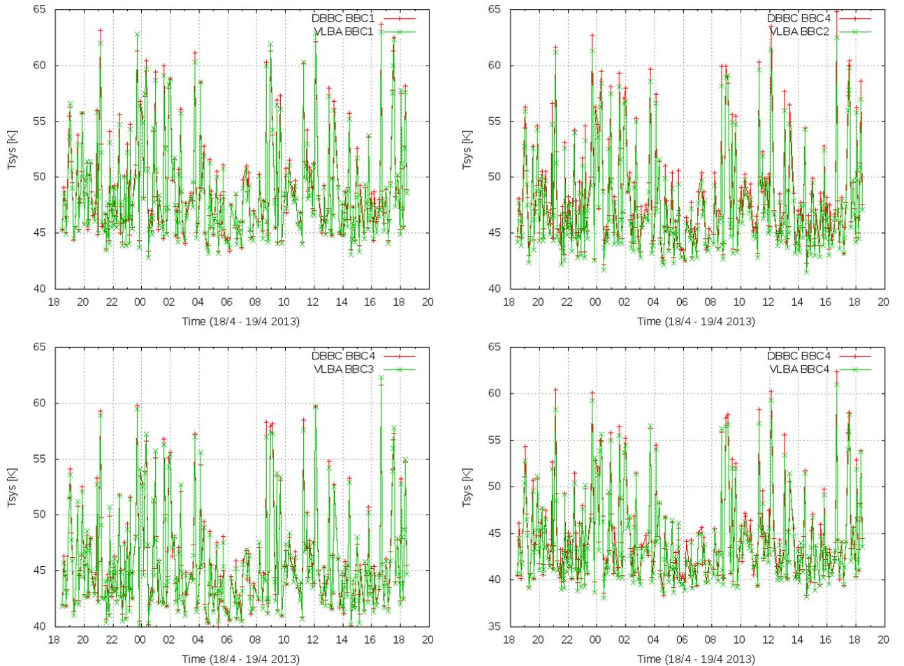
Figure 11: System temperature for IVS R4581 using the VLBA terminal and the DBBC in DDC mode (version 102) for BBCs 1 to 4.
