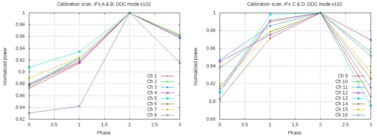
Figure 16: Calibration scan, DDC mode firmware 102. Normalized detected power versus time. IF was set to a manual level of 38000 counts and individual channels were set to manual. Left panel: RCP (IFA) and LCP (IFB), Right panel: RCP (IFC) and LCP (IFD)
