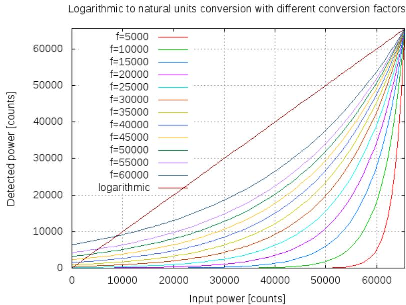
Figure 18: Conversion between logarithmic counts and linear counts with different factors
