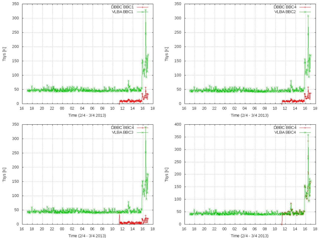
Figure 9: System temperature for IVS R1579 using the VLBA terminal and the DBBC in DDC mode (firmware version 103) for BBCs 1 to 4.
