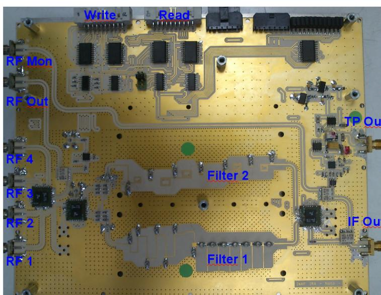
Figure 2: CoMo board (Unica 2 version). The detection power circuit is in the upper right corner of the board (to the left of the green dot sticker)
