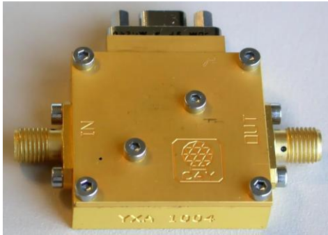
Amplifier external view.
