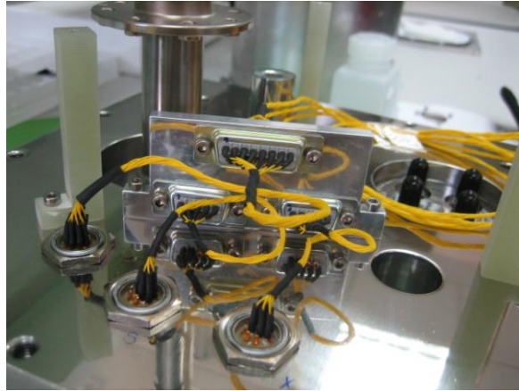
Figure 16: DC wiring (room temperature stage).
