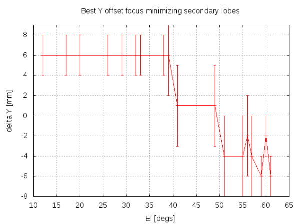
Figure 15: Best Y focus offset obtained from double pointing scans and minimizing the secondary lobe and maximizing the main beam intensity.
