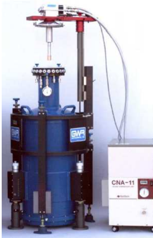
fig. 5 OSG dewar, vibration isolation frame and refrigerator
