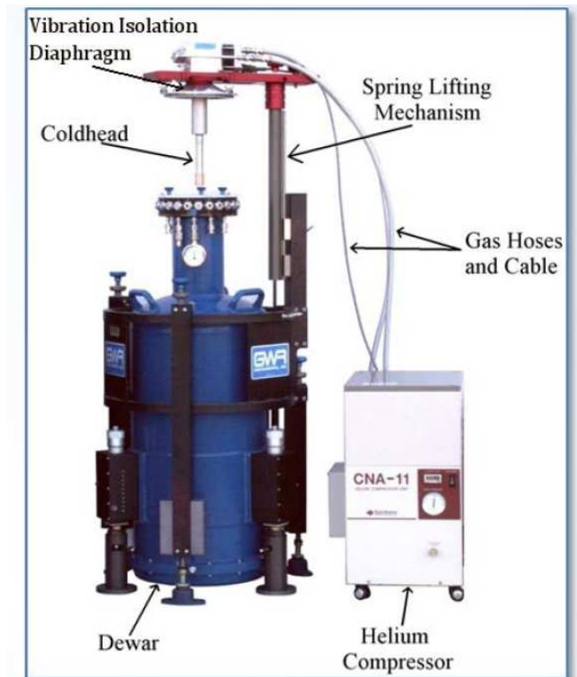
Figure 6: OSG Dewar and Refrigeration System shown with the coldhead lifted out of the dewar. The compressor is connected to the coldhead with flexible metal hoses and a power cable.
