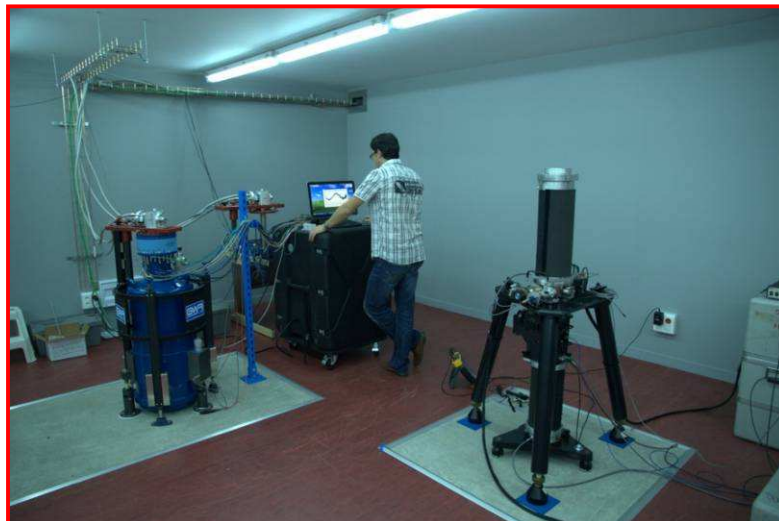
fig. 4 GWR-OSG and FG5 installed in Yebes
