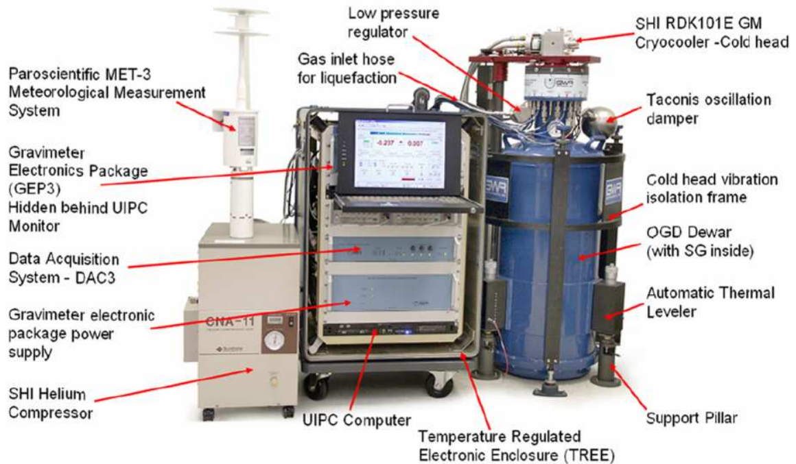
fig. 7. OSG subsystems
