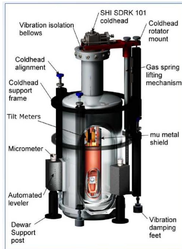
fig. 8 Cutaway view of dewar showing sensor mounted inside
