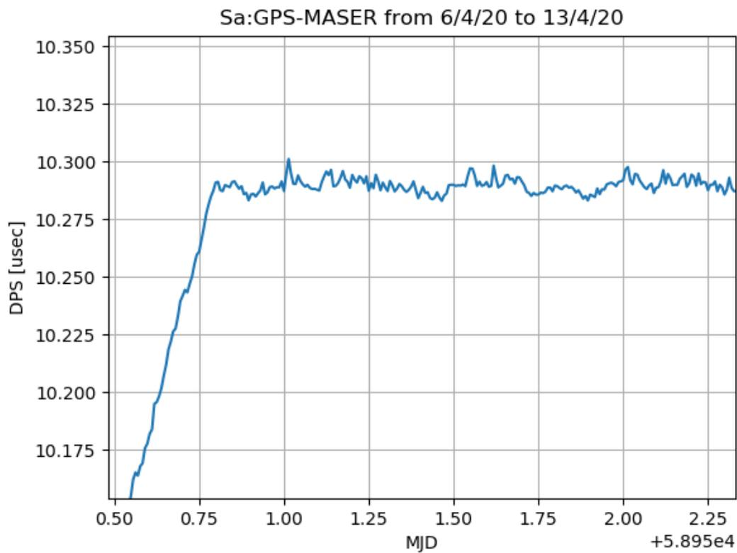
Figure 10: Syntonization on April 11th removed the frequency offset. Without the linear term, the noise becomes more evident.
