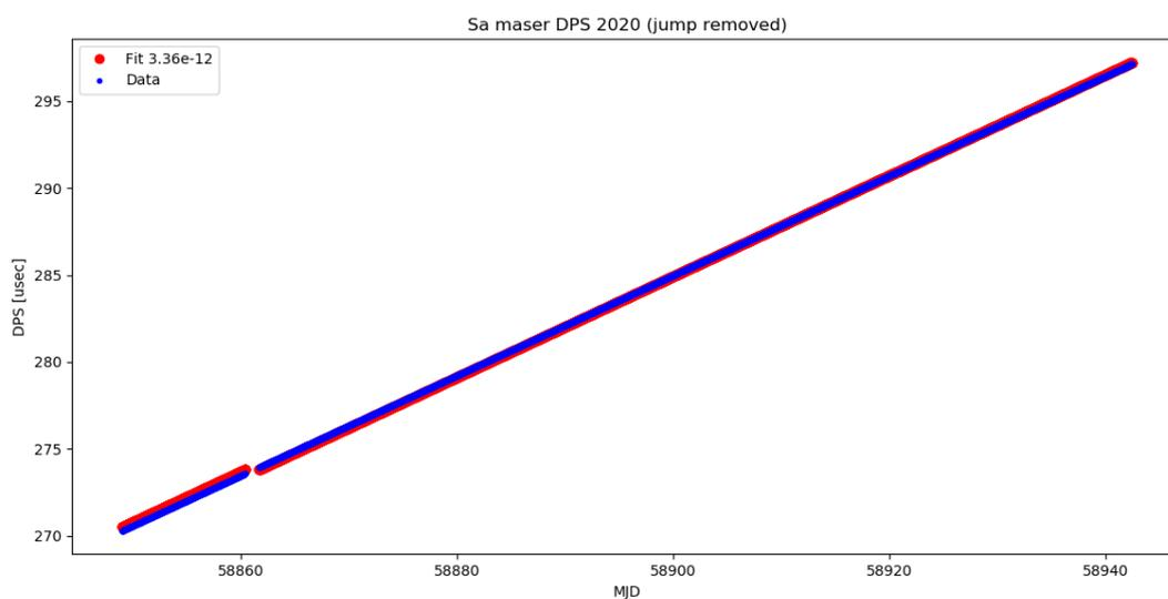
Figure 4: Linear fit to the DPS data after removing the synchronization jump. Notice the gap near  $MJD=58860$  that is now visible after changing the y domain range.
