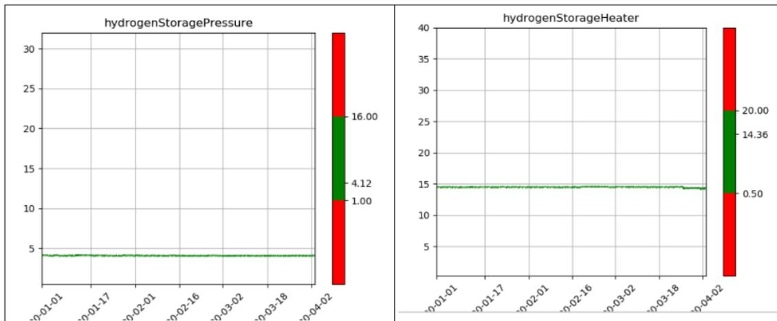
Figure 22: H storage monitoring parameters.
