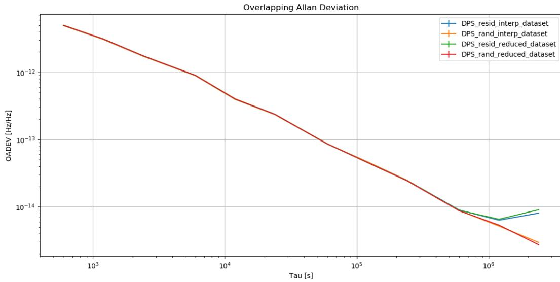
Figure 18: OADEV comparison for two different approaches to handle data with gaps.
