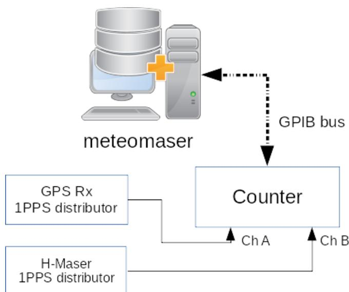
Figure 1: *Typical measurement setup.*
