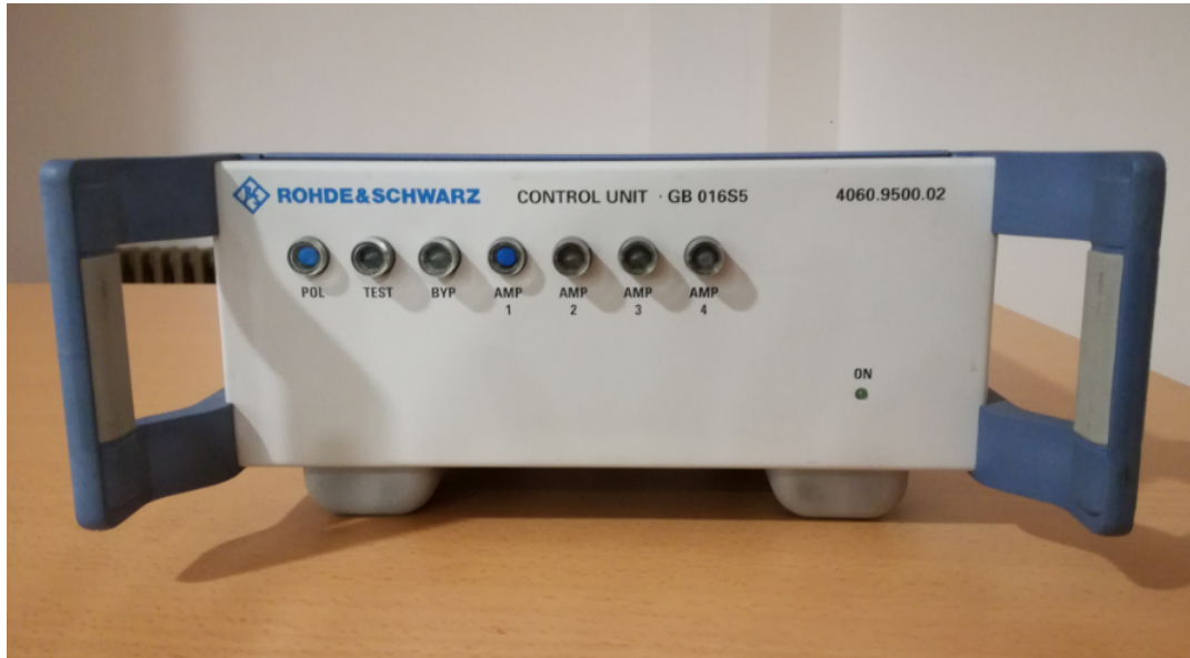
Figure 10: Front side of the control unit. In this case, amplifier 1 and vertical polarization are selected .
