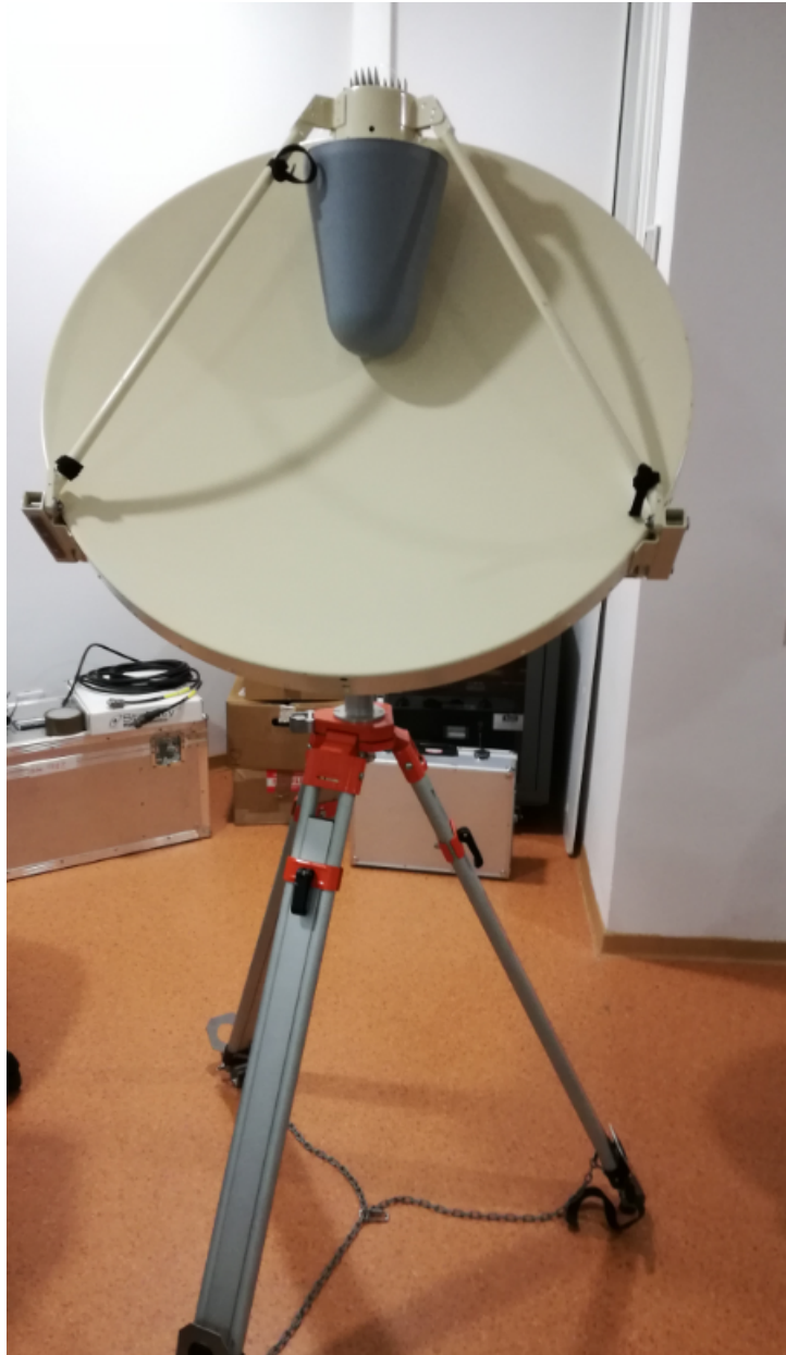
Figure 2: Parabolic antenna installed over the tripod.
